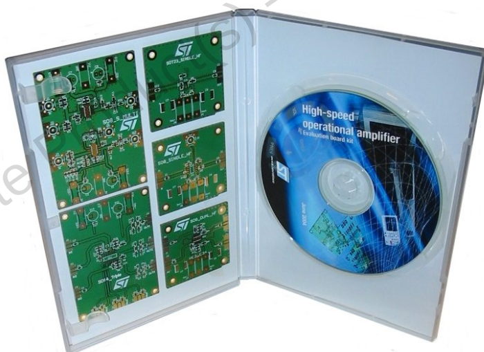
Figure 25: Evaluation kit for high-speed op-amps
