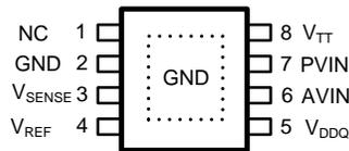
Figure 3. SO PowerPAD-8 (DDA0008A) Package Top View
