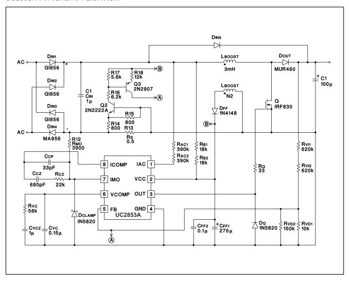
Note: the application circuit shown is a 100W, 63KHz design. Additional application information can be found in Application Note U–159 (TI literature Number SLUA080) and Design Note DN–78.
