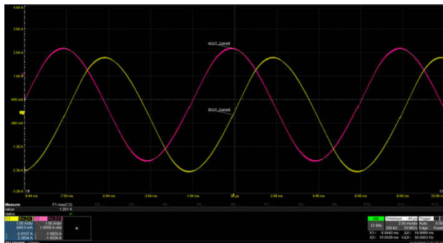
Figure 7-19. Coil Current Waveform with Silent Step Decay
