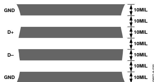
Figure 35. Arrangement of Signal Tracks
