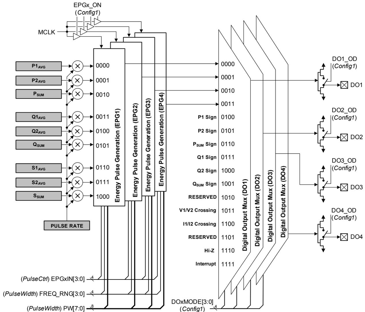
**Figure 14. Energy Pulse Generation and Digital Output Control**
