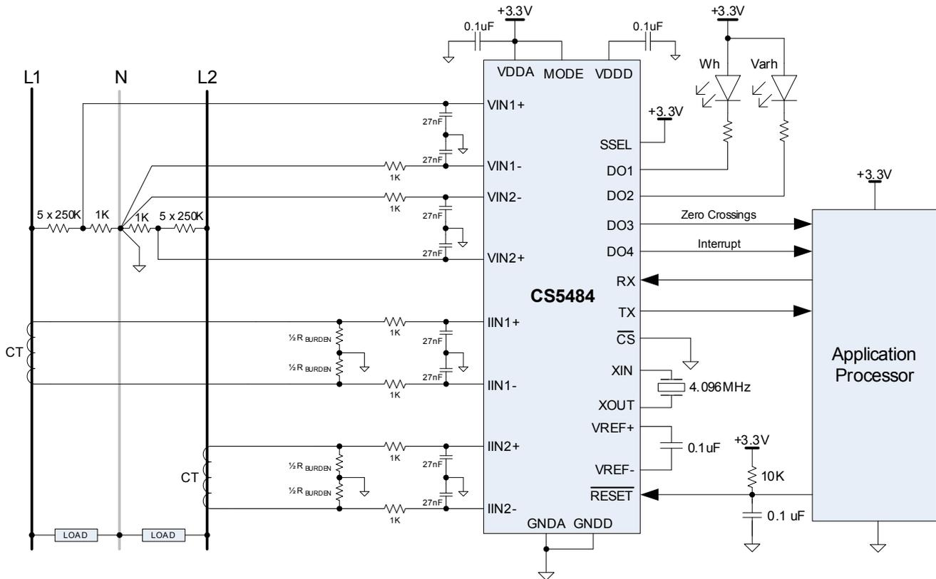
**Figure 25. Typical Connection (Single-phase, 3-wire, 12S Electricity Meter)**
