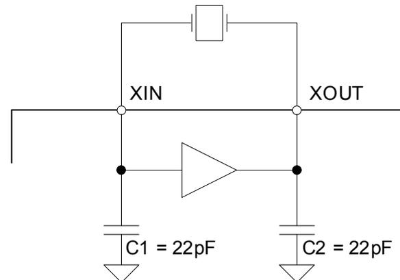
**Figure 1. Oscillator Connections**
