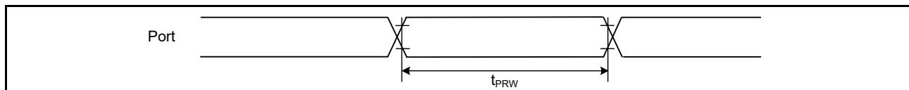
Figure 2.28 I/O ports input timing
