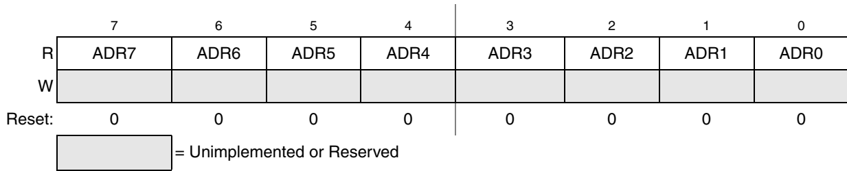
Figure 9-7. Data Result Low Register (ADCRL)
