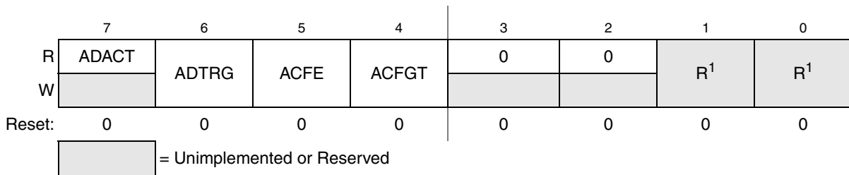
Figure 9-5. Status and Control Register 2 (ADCSC2)
