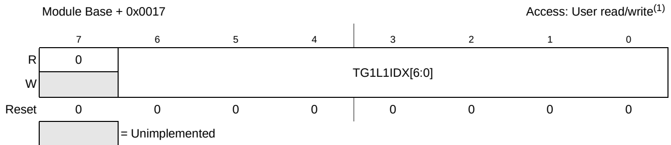
Figure 13-20. Trigger Generator 1 List 1 Index (TG1L1IDX)
