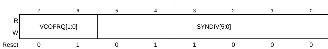
Figure 8-5. S12CPMU_UHV_V6 Synthesizer Register (CPMUSYNR)
