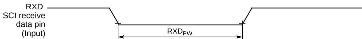
Figure 10-16 RXD Pulse Width
