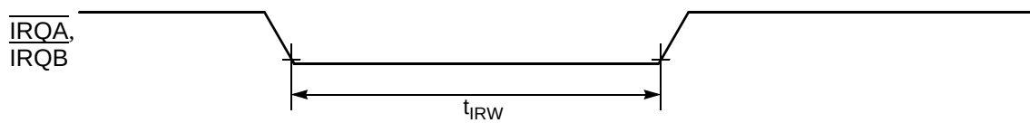
Figure 10-6 External Interrupt Timing (Negative Edge-Sensitive)
