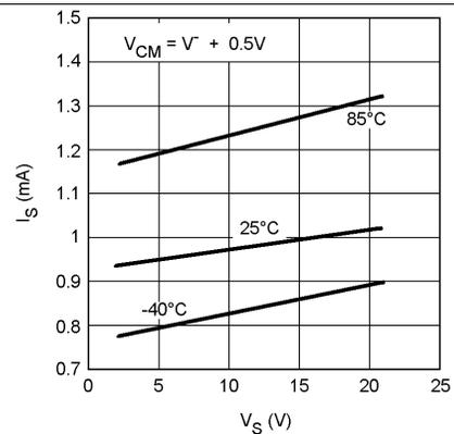
Figure 12. I<sub>S</sub> vs. V<sub>S</sub> (PNP side)
