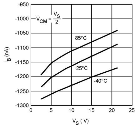
Figure 8. I<sub>B</sub> vs. V<sub>S</sub>
