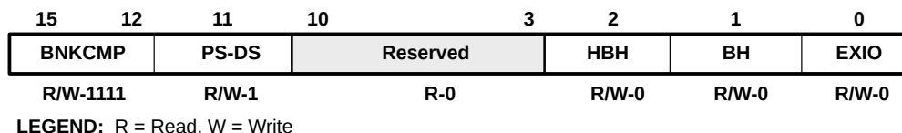
Figure 2–7. Bank-Switching Control Register (BSCR) [MMR Address 0029h]
