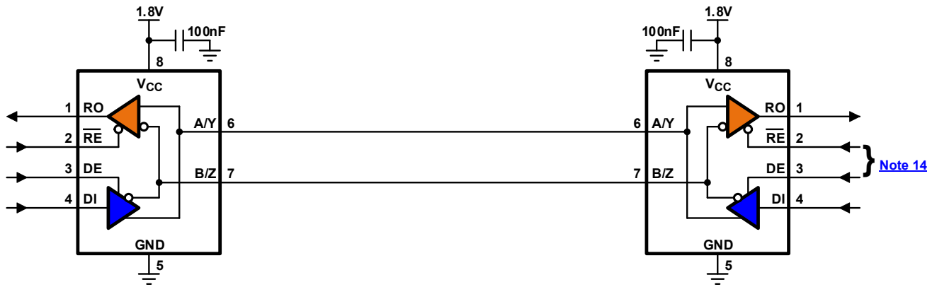
FIGURE 3. HALF DUPLEX NETWORK USING ISL32603E
