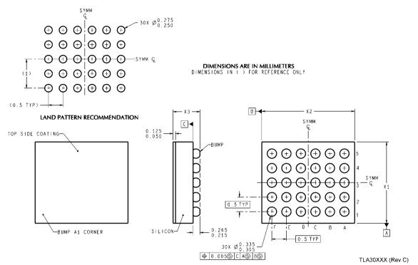
30-bump micro SMD Package NS Package Number TLA30D1A X1 = 2.568 mm ±0.030 mm X2 = 2.974 mm ±0.030 mm
