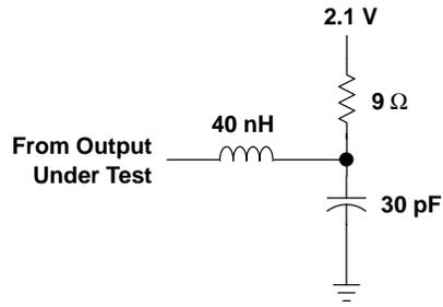
Figure 1. Load Circuit for  $V_{OHP}$  and  $V_{OHV}$
