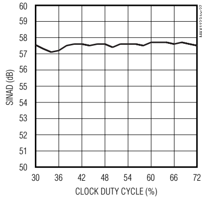
SINAD vs. CLOCK DUTY CYCLE ( f_{IN} = 1.4106MHz , f_{SAMPLE} = 210.0428MHz , A_{IN} = -0.5dBFS )
