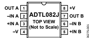
Figure 1. 8-Lead SOIC_N (R-8)
