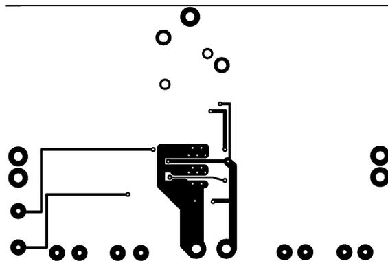
Figure 50. Recommended MTE PC Board Layout: Bottom-Side Layout
