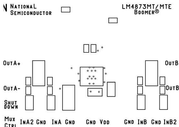
Figure 48. Recommended MTE PC Board Layout: Component-Side Silkscreen
