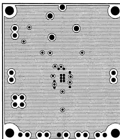
Figure 55. Recommended LQ PC Board Layout: Bottom-Side Layout
