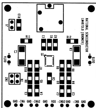
Figure 51. Recommended LQ PC Board Layout: Component-Side Silkscreen
