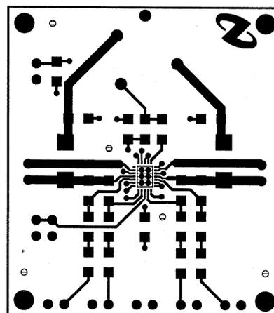
Figure 52. Recommended LQ PC Board Layout: Component-Side Layout
