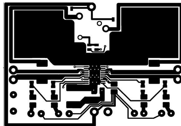
Figure 49. Recommended MTE PC Board Layout: Component-Side Layout
