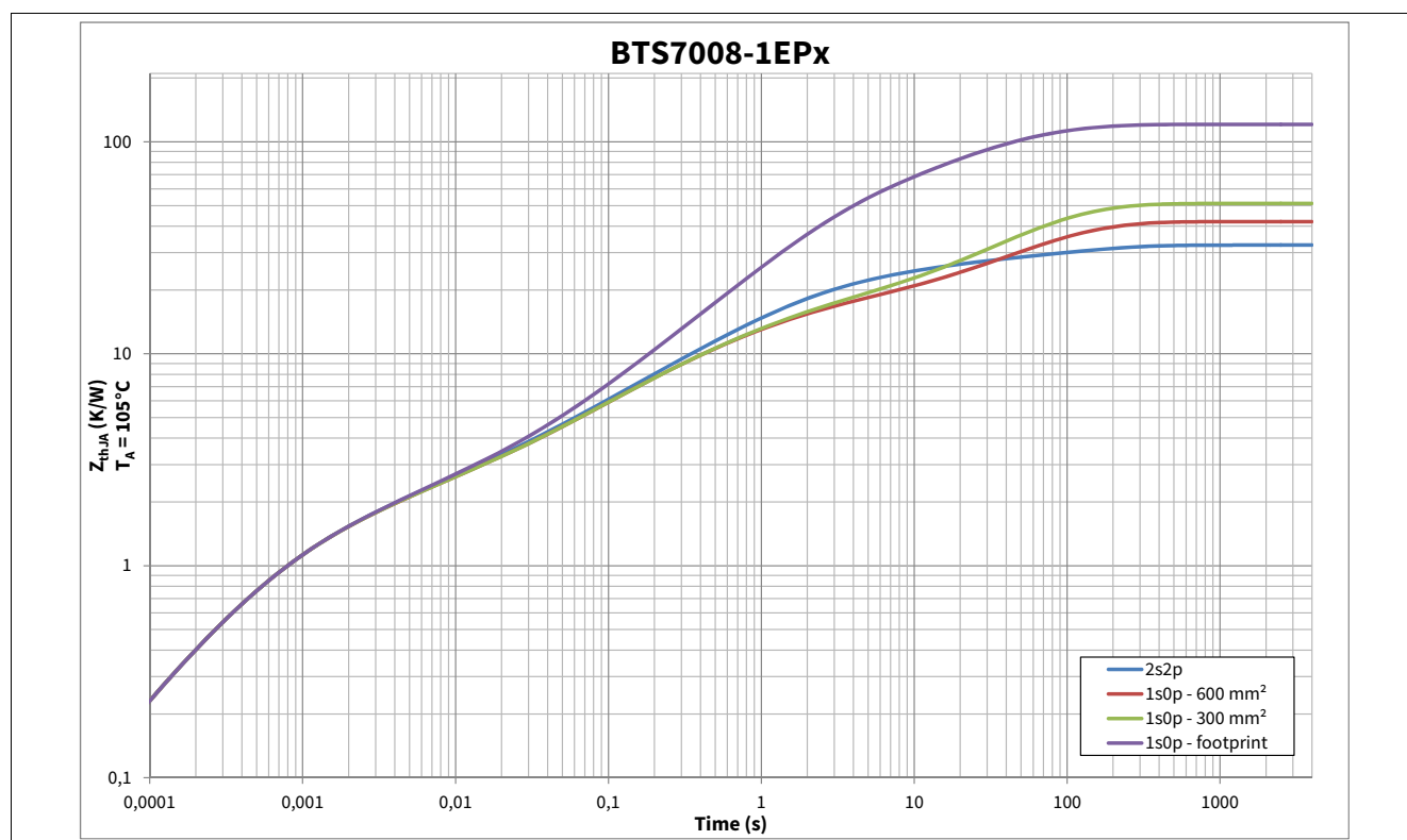
Figure 9 Typical Thermal Impedance. PCB setup according Chapter 4.4.1
