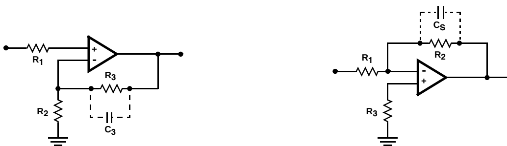
FIGURE 3. SUGGESTED OFFSET VOLTAGE ADJUSTMENT
