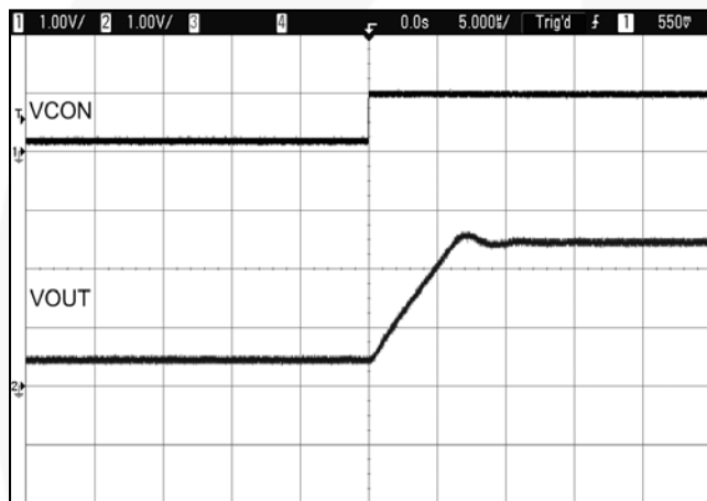
Figure 36. V_{OUT} Rising Transition 0.5 V to 2.5 V, V_{IN} = 3.7\text{ V} in Low-Power Mode
