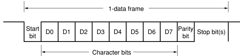
Figure 16-7. Format of Asynchronous Serial Interface Transmit/Receive Data
