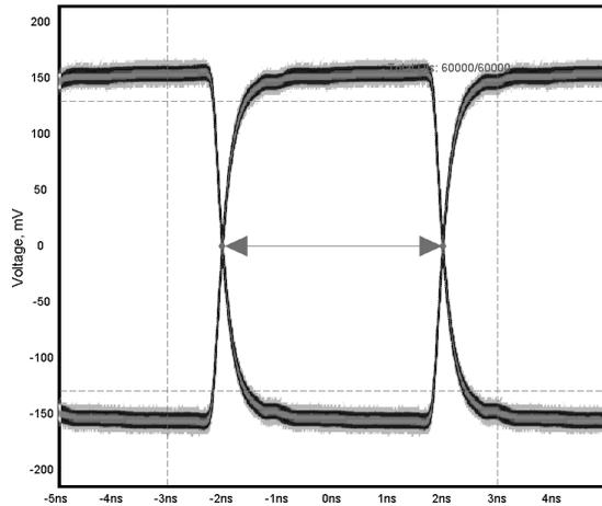
**Figure 15. LVDS RxCLKOUT Output**
