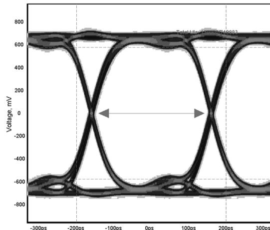
**Figure 20. Retimed Loop Through Output**
