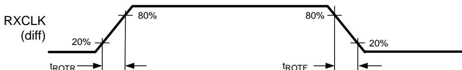
Figure 4. LVDS Output Transition Time
