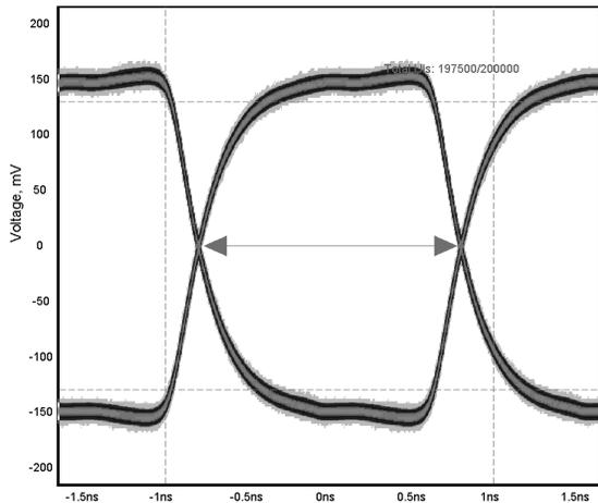
**Figure 17. LVDS RxCLKOUT Output**
