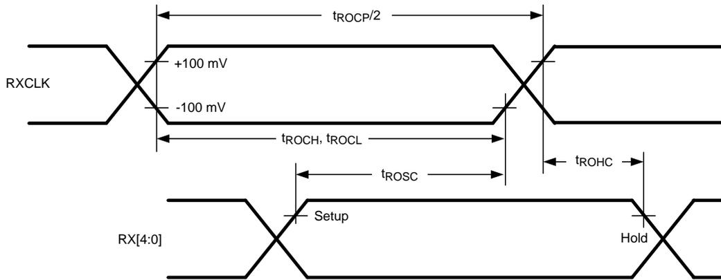
**Figure 5. Deserializer (LVDS Interface) Setup/Hold and High/Low Times**
