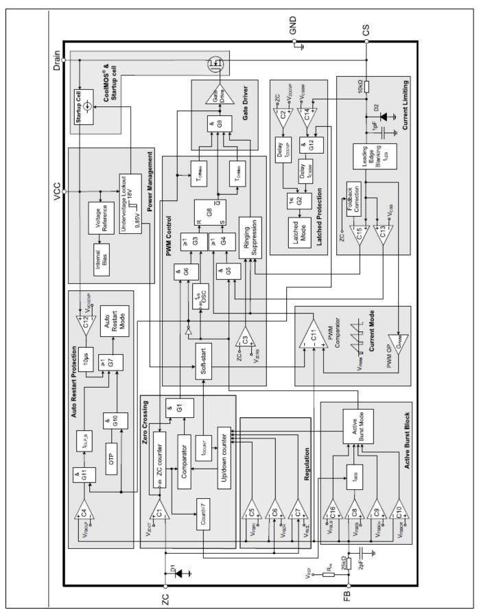
Figure 3 Representative Block Diagram
