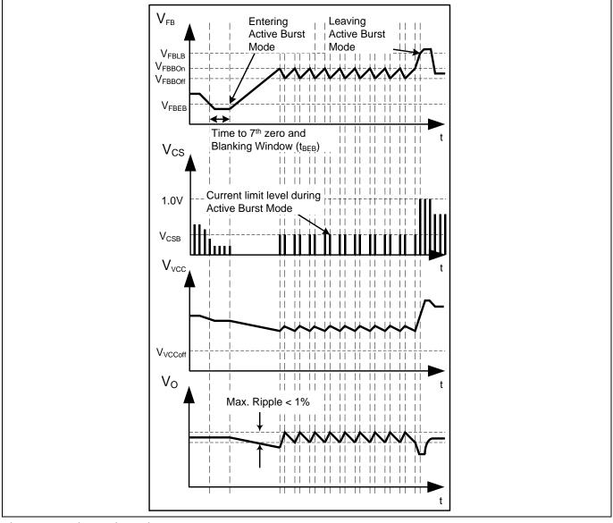
Figure 9 Signals in Active Burst Mode
