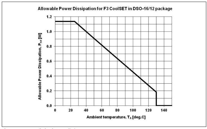
Figure 11 Power dissipation; Ptot=f(Ta)
