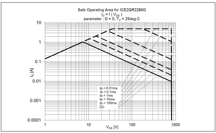
Figure 10 Safe Operating Area (SOA) curve for ICE2QR2280G-1
