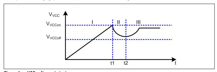
Figure 4 VCC voltage at start up
