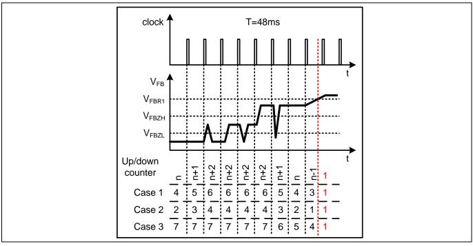
Figure 6 Up/down counter operation
