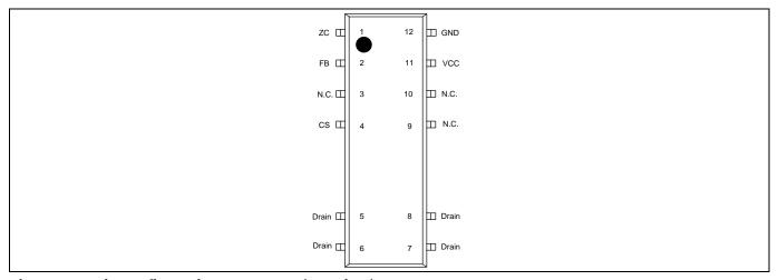
Figure 2 Pin configuration PG-DSO-12(top view)
