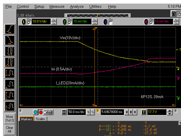
FIGURE 15. LINE REGULATION WITH V_{IN} CHANGE FROM 26V TO 6V FOR 4P12S AT 20mA/CHANNEL
