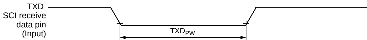
Figure 10-16 TXD Pulse Width
