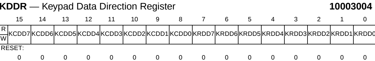
Figure 14-4 Keypad Data Direction Register
