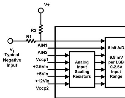
Resistor values shown in Table 2 provide approximately 1.25V at the Vccp inputs.
