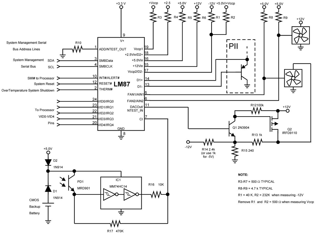
In this PC application the LM87 monitors temperature, fan speed for 2 fans, and 6 power supply voltages. It also monitors an optical chassis intrusion detector. The LM87 provides a DAC output that can be used to control fan speed.
