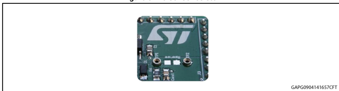
Figure 4: Mounting through-hole sense resistor
