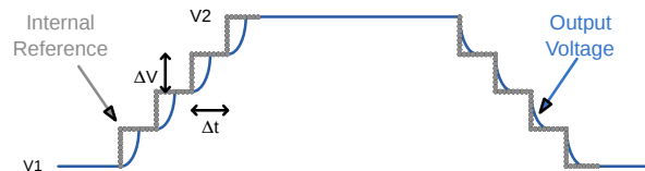
Figure 44. DVS in Forced PPWM Mode Diagram
