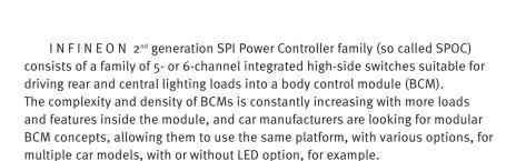
The SPOC II family, scaled by number of channels and features (basic, LED mode, cranking), addresses this trend and integrates multiple channels inside one package to reduce board space. SPOC II devices feature a serial peripheral interface (SPI), enabling customers to save I/Os in the microcontroller and reduce the amount of external components required for a discrete implementation. The LED mode in BTS5672E and BTS5682E is programmable via SPI.
