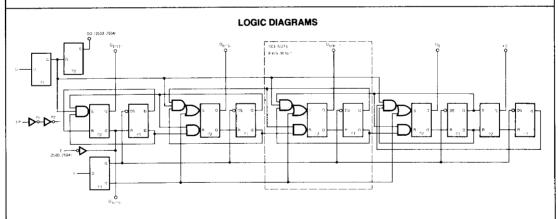
Notes: 1. Cell logic is repeated for register stages.  $Q_5$  to  $Q_1$  Am2502/3,  $Q_9$  to  $Q_1$  Am2504.
