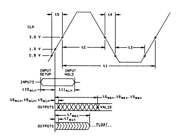
FIGURE 4. Timing waveforms.
