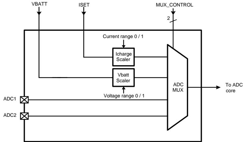
The source selection and the access to the conversion results are established through the I<sup>2</sup>C linked control registers: ADCC and ADCD as described below:
