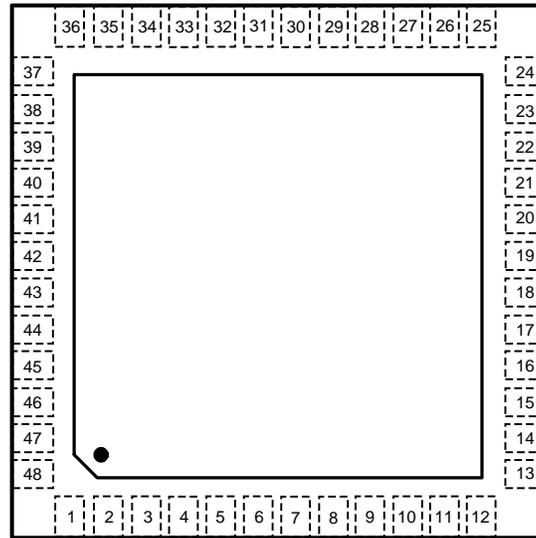
Figure 2. 48 WQFN Package (Top View)
