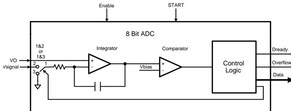
The A/D converter multiplexes 4 different sources:
