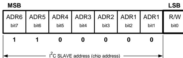
Figure 63. I<sup>2</sup>C Write Cycle
