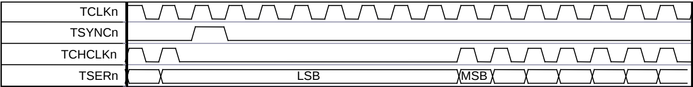
Figure 11-31. E1 Transmit-Side TCHCLKn Gapped Mode During Channel 1
