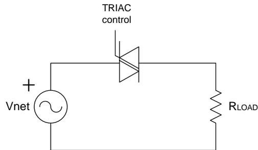
The firing angle ( $\alpha$ ) of the switch can be varied. The average voltage will be proportional to the area under the sine wave. Thus, the average voltage is the integral from the firing angle to the zero crossing.
