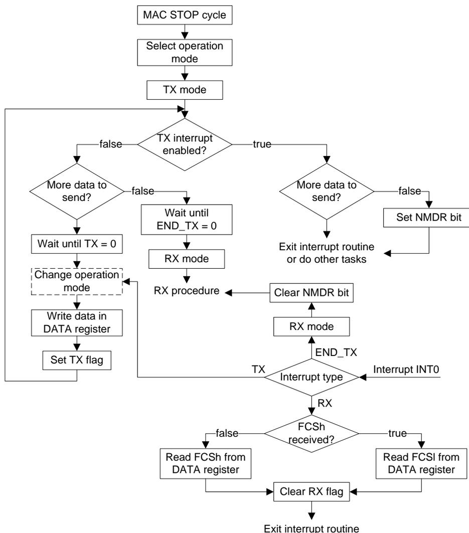
At the beginning of the procedure, the MCU must configure the MAC in transmission mode and select the desired operation mode.
