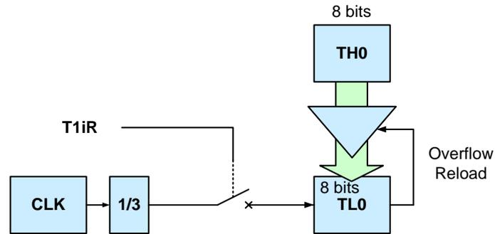
Timers T1i count machine cycles (3 clock cycles) in normal operation mode. They can be forced to count clock cycles. To enter this mode the corresponding bits in T1NP register must be set to '1' (T1NP(i-1) controls T1i). Unused bits in T1NP, bits 4 to 7, are not defined. Writing to these bits has no effect, reading these bits will always get "0000".
