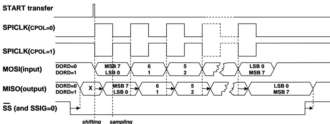
Note that the master selects a slave by driving the slave select pin of the corresponding slave device. Data written to the SPDAT register of the master is shifted out of the MOSI pin of the master to the MOSI pin of the slave, at the same time the data in SPDAT register on slave side is shifted out on its MISO pin to the MISO pin of the master.
