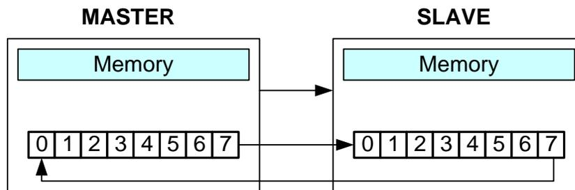
If SPEN = 1, SSIG = 0 and MSTR = 1, the SPI0 is enabled in master mode. The SS pin is quasi-bidirectional. In this case, another master can drive this pin low to select this device as an SPI slave and start sending data to it. To avoid bus contention, the CPU becomes a slave. As a result of the observed SPI module becoming a slave, the MOSI and SPICLK pins are forced to be an input and MISO becomes an output.
