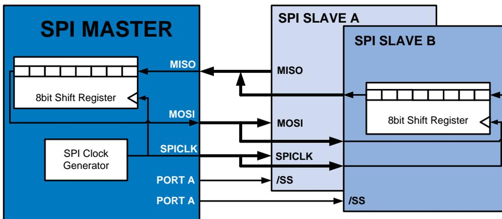
In Figure 7-5, slave's SSIG = 0, and SS is used to select the slave. The SPI0 master can use any port pin (including P5.0/SS with SSIG = 1) to drive the SS pin.
