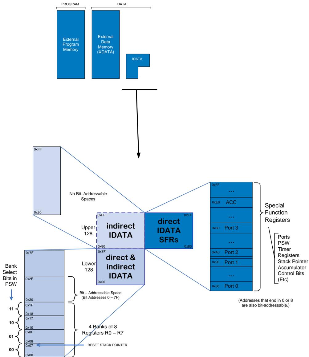
Logical addressing of the Internal Data Memory is mapped as shown in Figure 4-8. The internal IDATA memory space has a total size of 384 bytes and is divided into three blocks, which are generally referred to as the Lower 128 bytes, the Upper 128 bytes and SFR space (128 bytes size).
