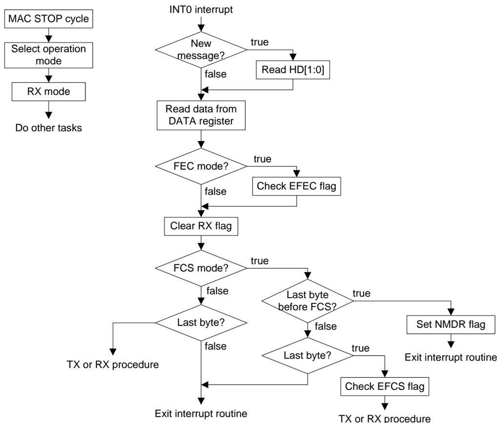
For each processed byte, an interrupt alerts the MCU. If the FLAGS1[RxFEC] bit is set, then FEC fields are also passed to the MCU via the interrupt method. If the message includes error protection and/or detection mechanism, the MAC hardware uses the flags FLAGS2[EFEC] and FLAG2[EFCS] to inform about the computation results. However, it is a MCU decision to abort the reception process or not. The reception of the message can be aborted anytime by issuing a STOP cycle.
