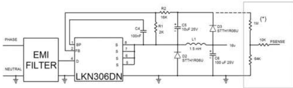
\*This Resistor must support high voltages
