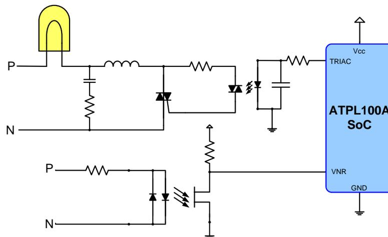
To connect a mains switch to the integrated circuit, an optocoupled connection is the preferred option (see [Figure 9-8](#)).
