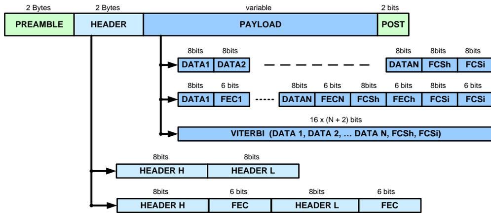
A standard packet encapsulation has the following structure
