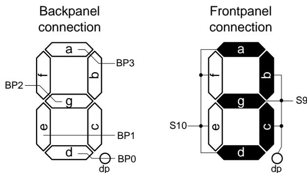
The above segment assignments are provided by the specification of the LCD glass for this example. Segment assignments according to this specification are shown below:
