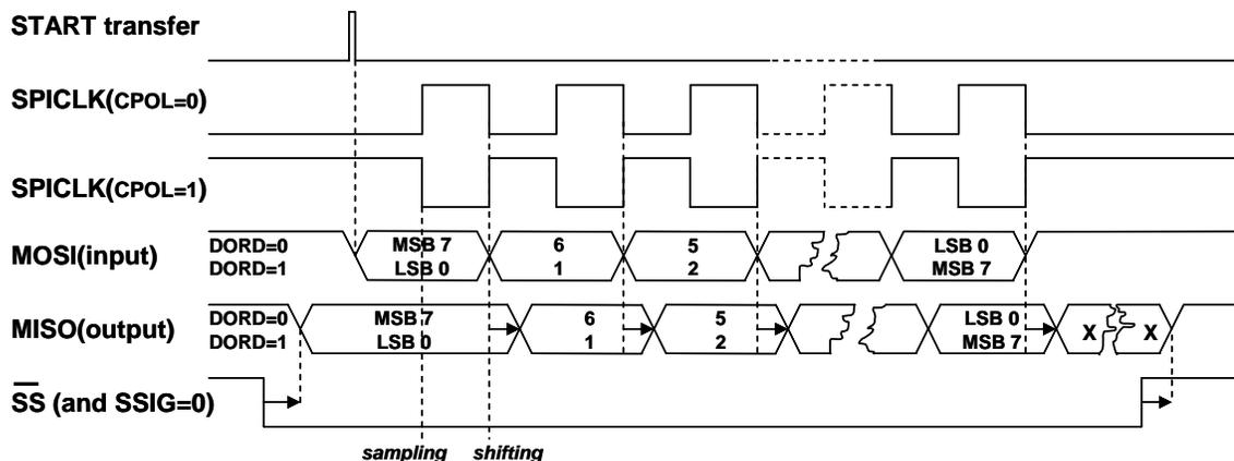
Figure 7-3. SPI0 transfer with CPHA=1
