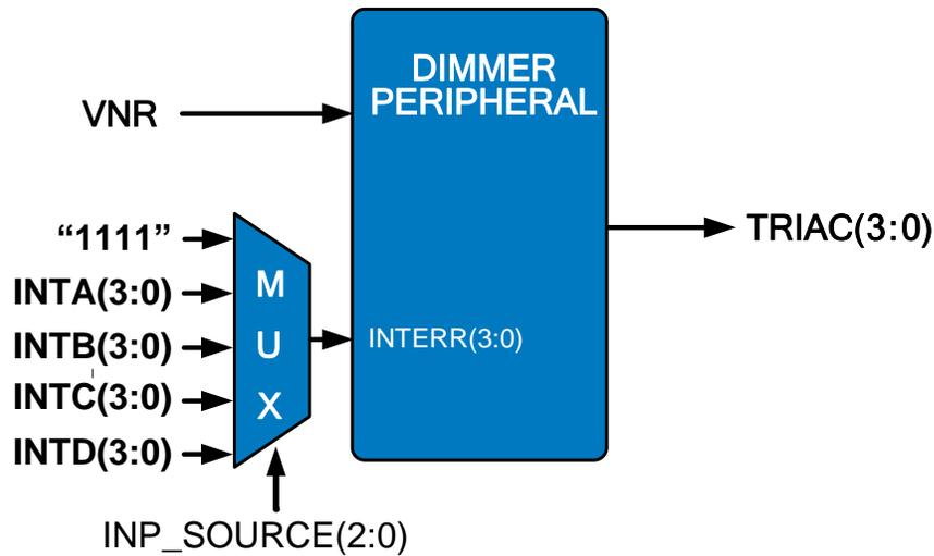
This peripheral is capable of doing a Phase Angle control in order to change the power of the loads. Phase Angle control uses a low switch frequency to chop the power line sine wave.
