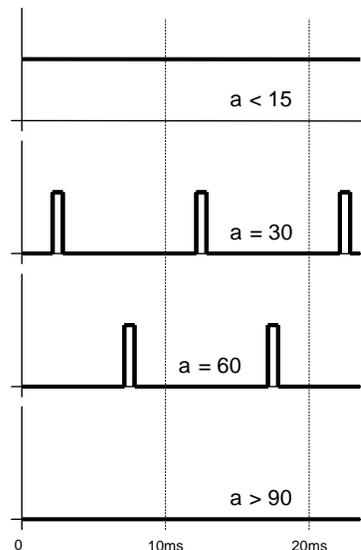
**In case that PWM mode is selected**, these four registers are used to adjust the duty cycle. In this case, each one must contain a value between 0 and 255 (0xFF). When 255 (0xFF), PWM output is always VDD.
