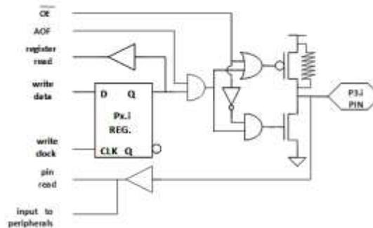
Figure 4-14. Pins without AOF structure
