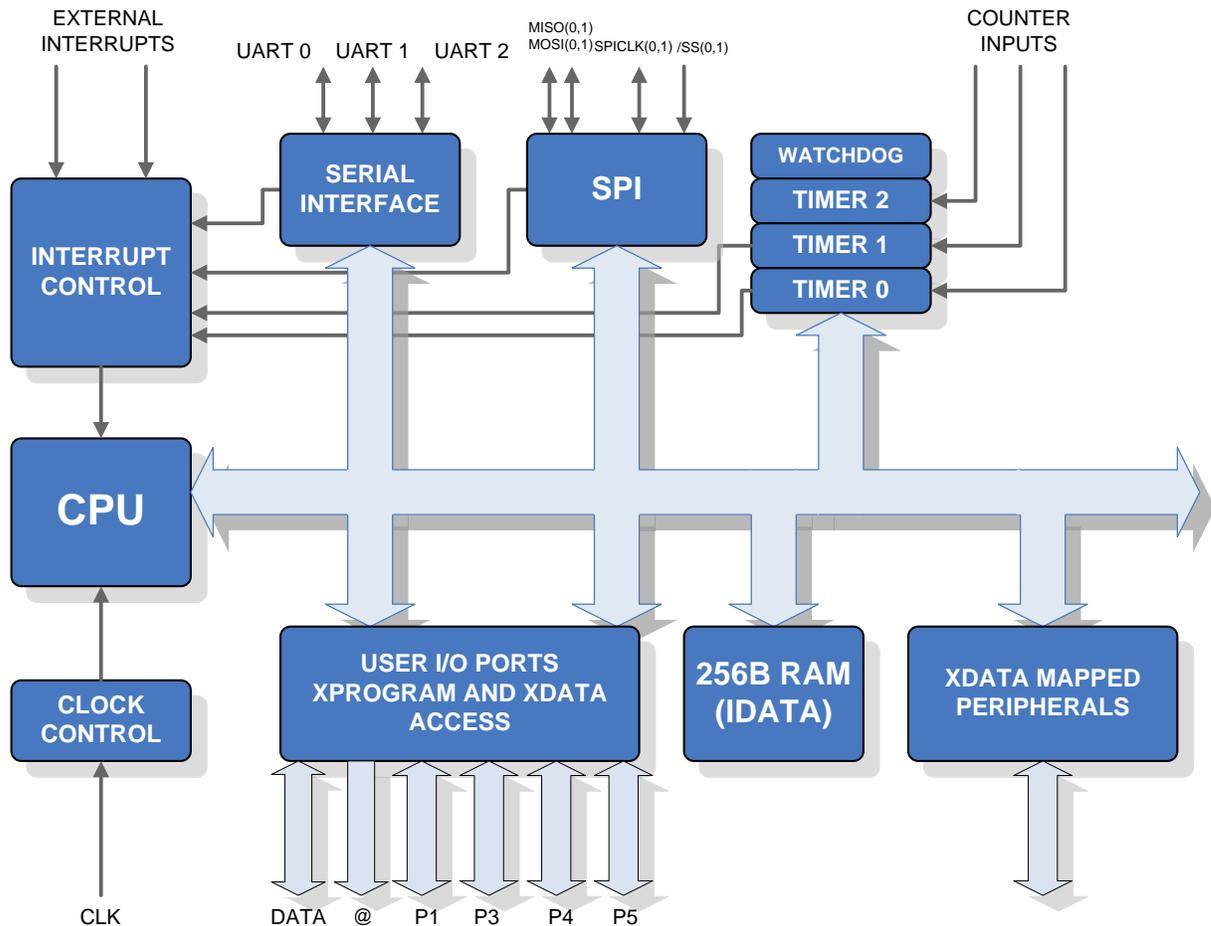
Note: This chapter describes the architecture from the microcontroller point of view. Thus, “on-chip SRAM” is referred to as “external memory” since “external” instructions like MOVX are necessary to access this memory device
