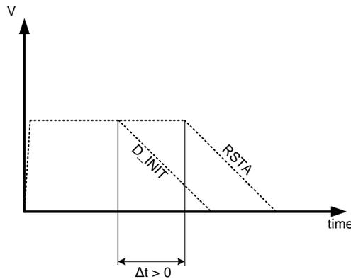
Not minimum time is required between both releases,  $\Delta t > 0$ , so a simple RC circuit is enough to satisfy this requirement.
