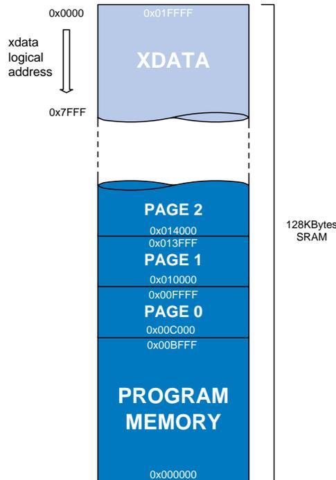
Common and extended memory sizes vary depending on the value in P0(7:6), as shown above. According to these size values, the core knows when the PC is pointing to an address located in common memory and when it is pointing to an address located in extended memory. When PC is pointing to an address in extended memory, then P0(5:0) indicates the extended page number and the physical address is automatically calculated. Some examples are shown below.
