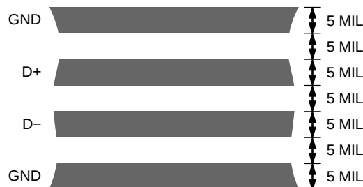
Figure 34. Typical Arrangement of Signal Tracks
