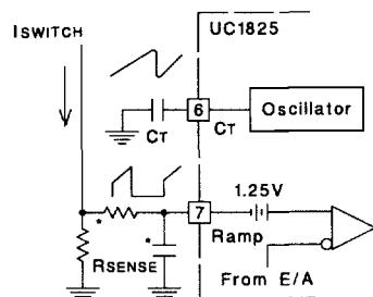
\* A small filter may be required to suppress switch noise.
