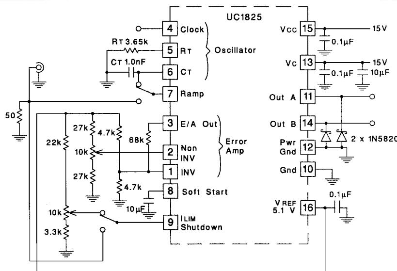
This test fixture is useful for exercising many of the As with any wideband circuit, careful grounding and bypass procedures should be followed. The use of a ground plane is highly recommended.
