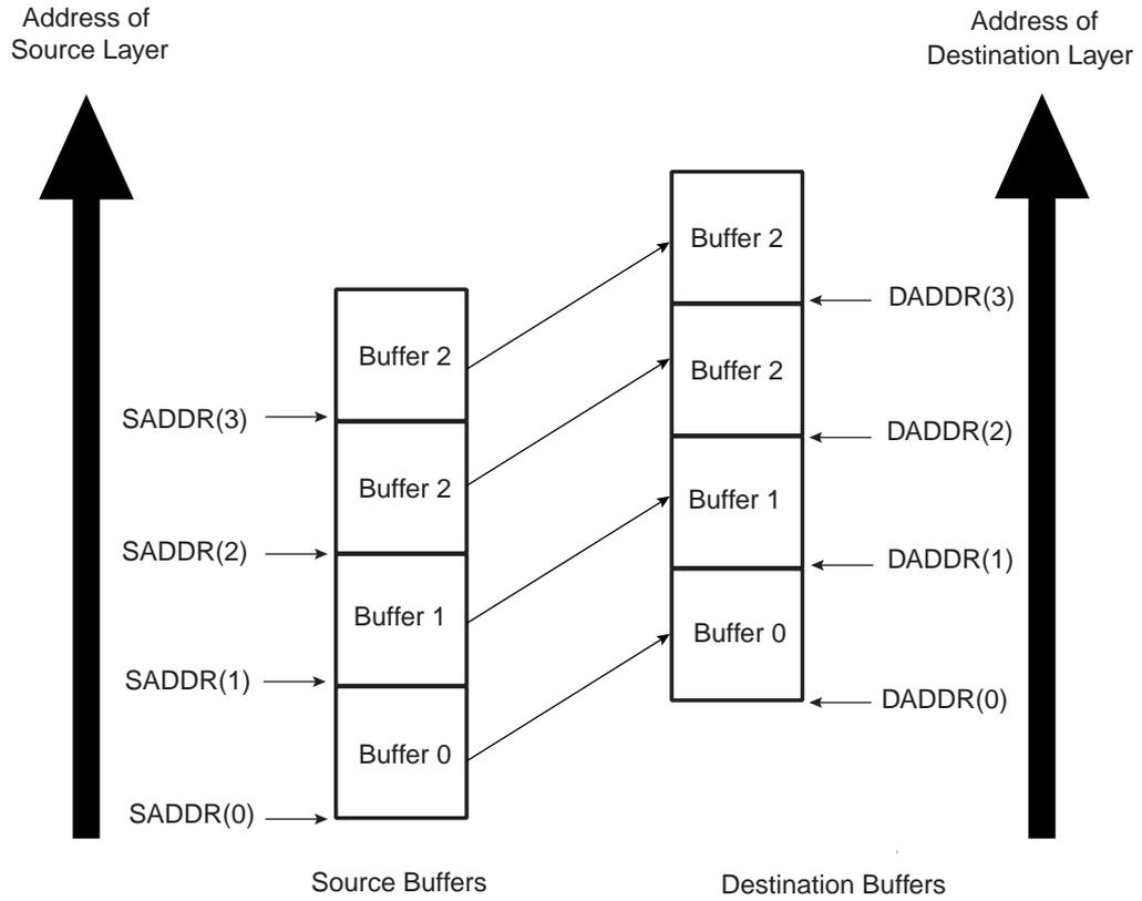
The DMAC transfer flow is shown in [Figure 40-8 on page 985](#).
