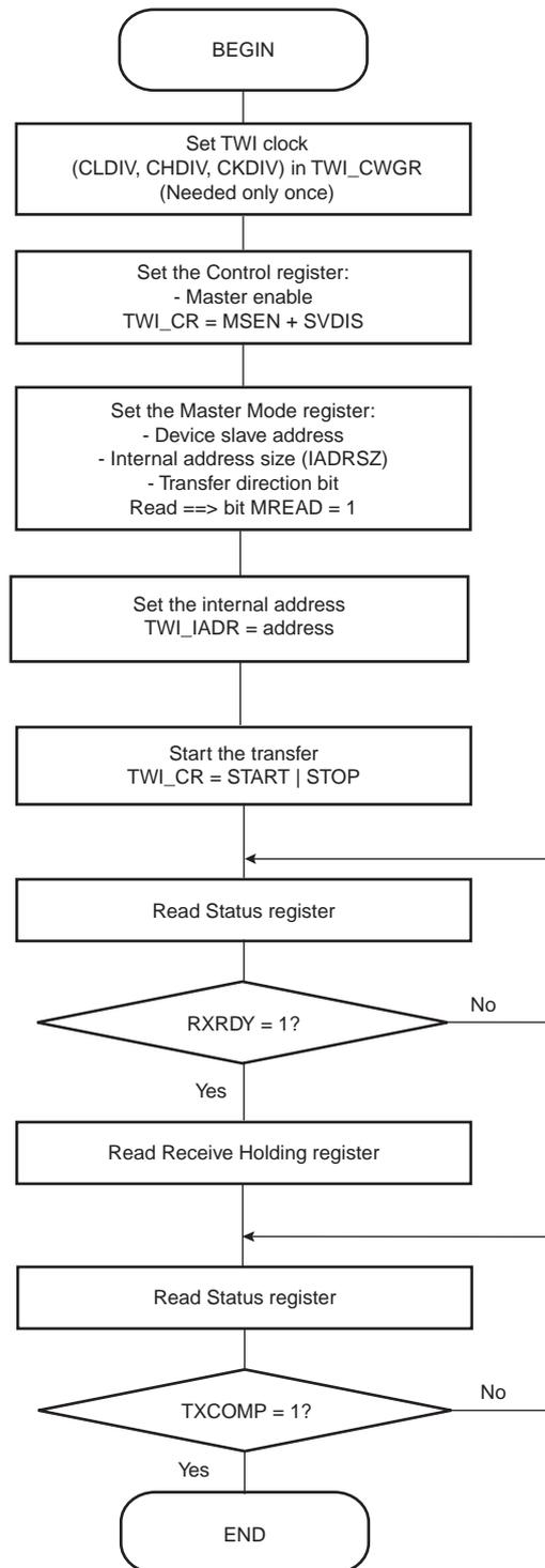
Figure 30-20. TWI Read Operation with Multiple Data Bytes with or without Internal Address
