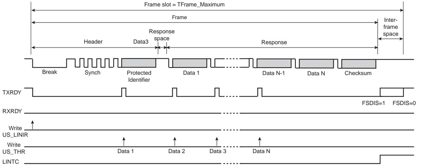
**Figure 32-47. Master Node Configuration, NACT = SUBSCRIBE**
