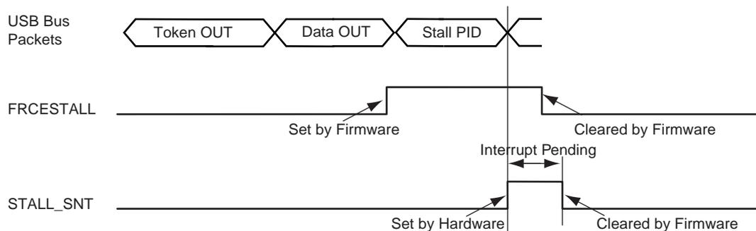
**Figure 37-17. Stall Handshake Data IN Transfer**
