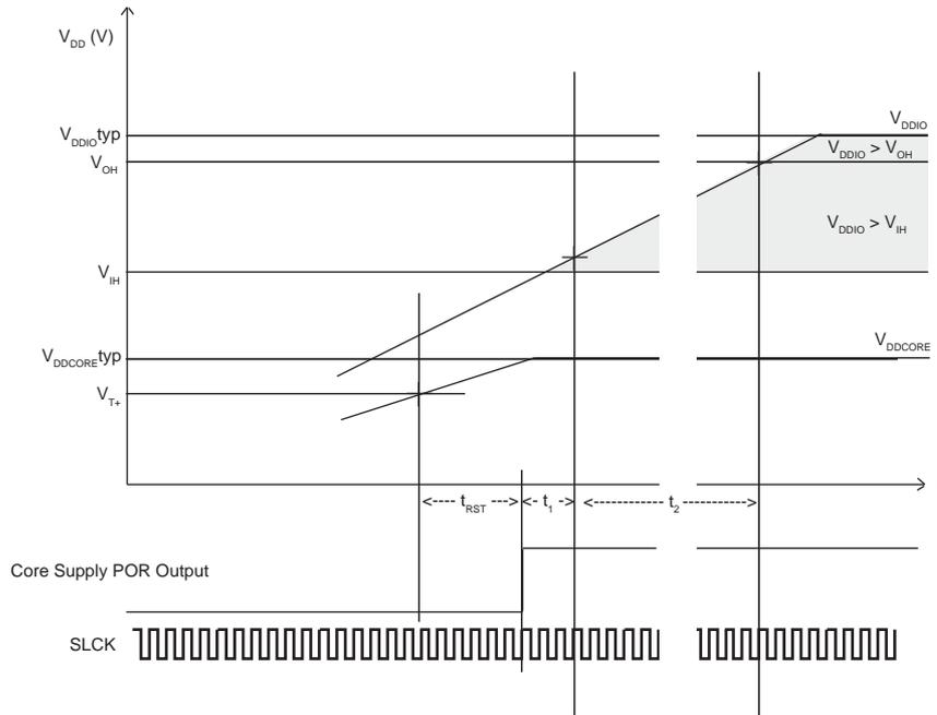
$V_{DDCORE}$  and  $V_{DDBU}$  are controlled by the internal PORs (Power-on Reset) to guarantee that these power sources reach their target values prior to the release of POR.
