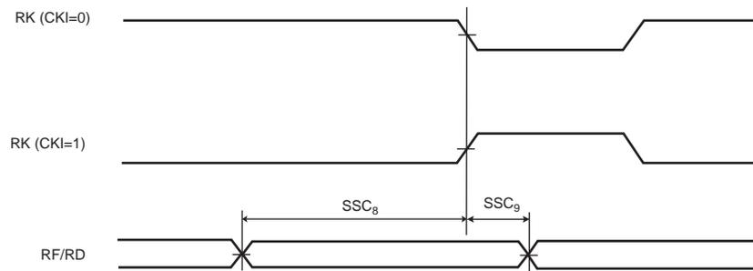
**Figure 48-17. SSC Receiver, RK in Input and RF in Output**
