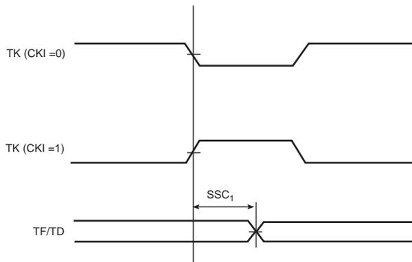
**Figure 48-15. SSC Transmitter, TK in Output and TF in Input**
