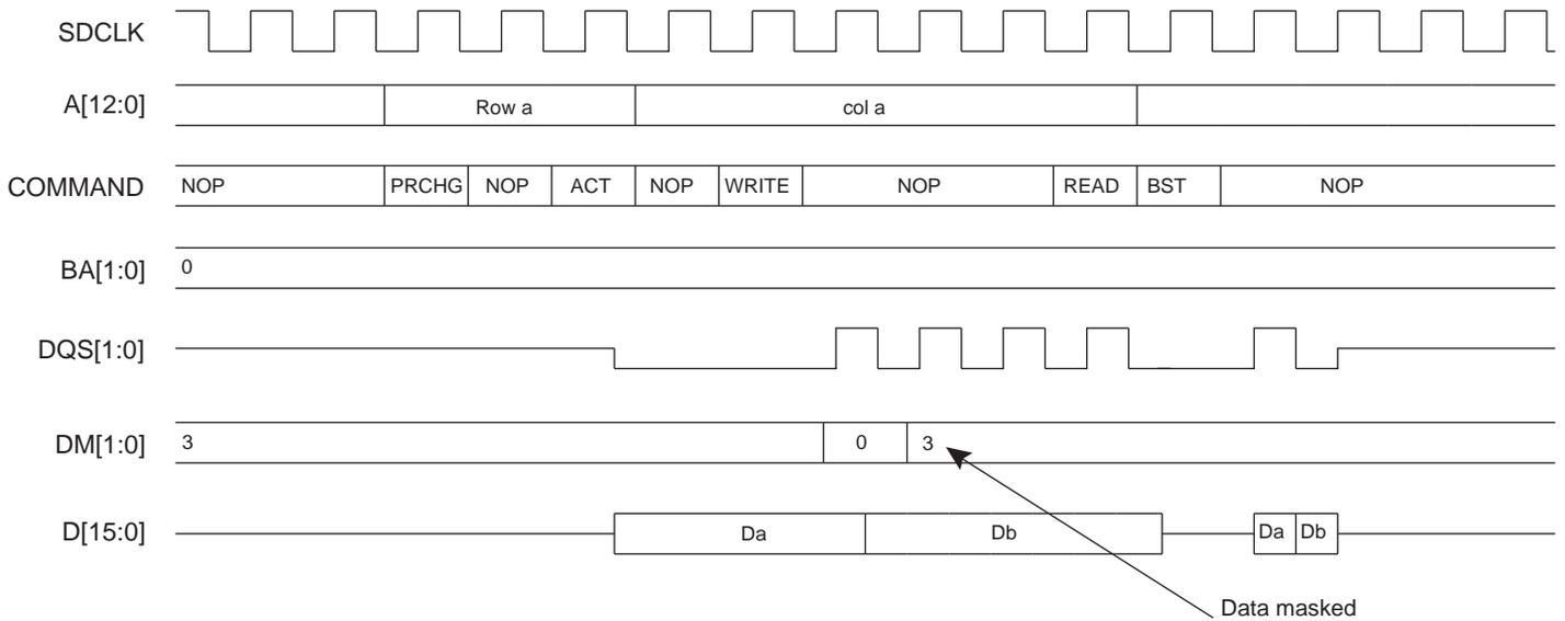
**Figure 21-10. SINGLE Write Access Followed By A Read Access, DDR2 -SDRAM Device**
