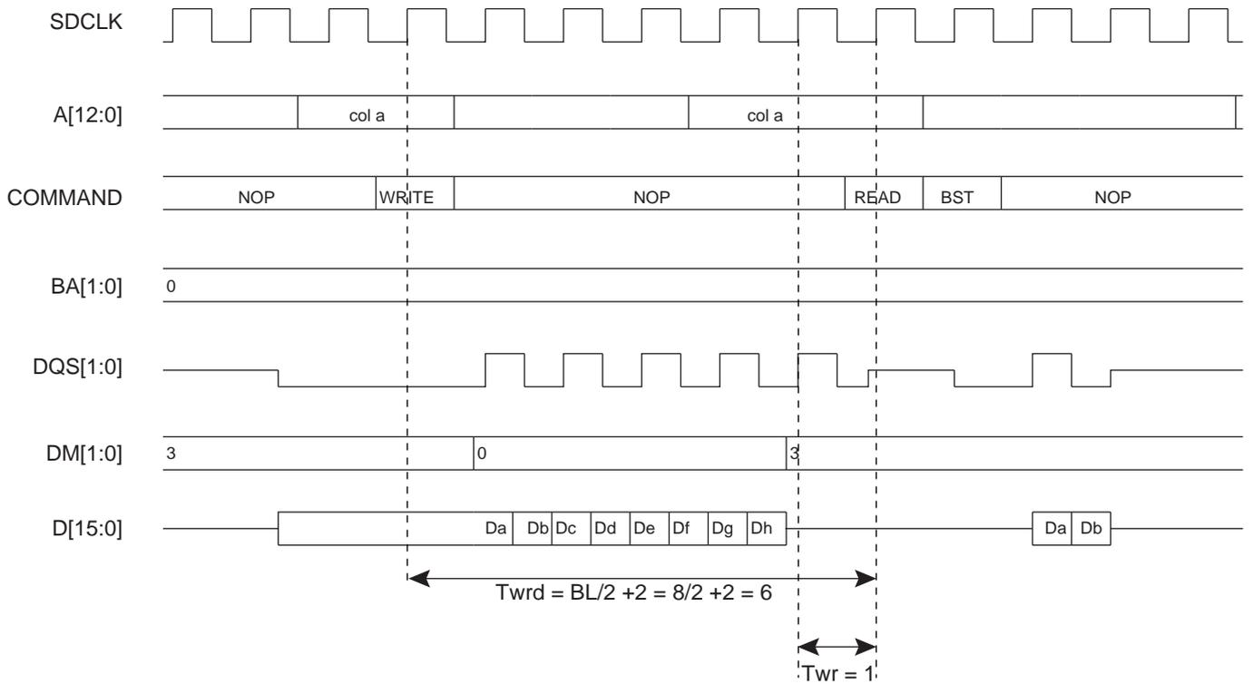
In the case of a single write access, write operation should be interrupted by a read access but DM must be input 1 cycle prior to the read command to avoid writing invalid data. See [Figure 21-9](#).
