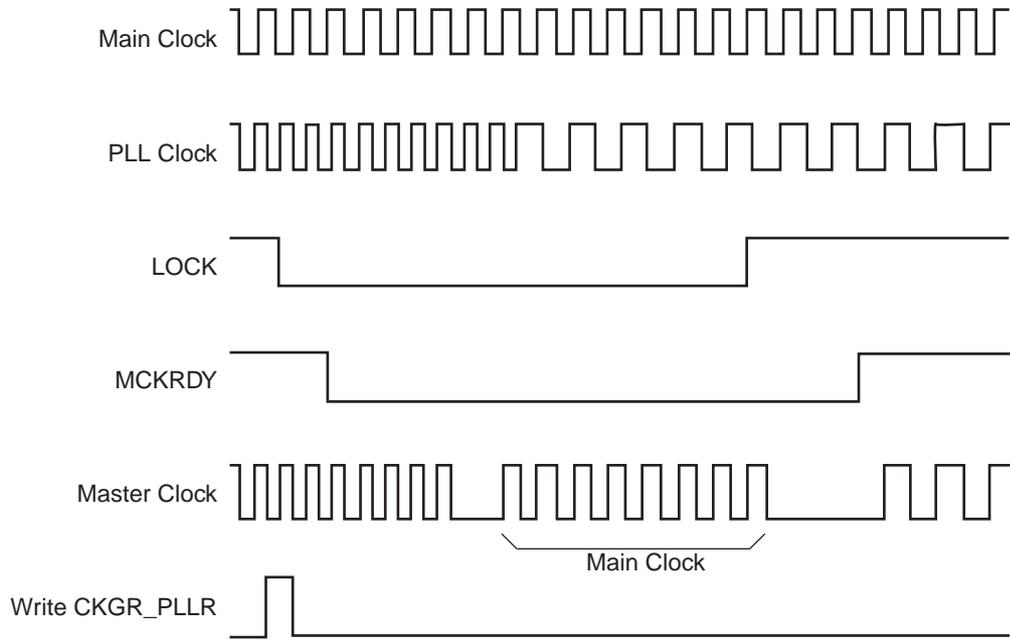
**Figure 25-6. Programmable Clock Output Programming**
