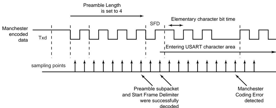
When the start frame delimiter is a sync pattern (ONEBIT field at 0), both command and data delimiter are supported. If a valid sync is detected, the received character is written as RXCHR field in the US\_RHR and the RXSYNH is updated. RXCHR is set to 1 when the received character is a command, and it is set to 0 if the received character is a data. This mechanism alleviates and simplifies the direct memory access as the character contains its own sync field in the same register.
