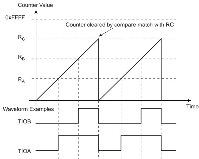
**Figure 31-10. WAVSEL = 10 With Trigger**
