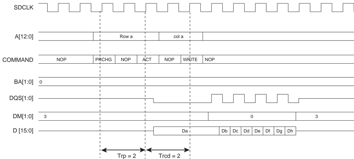
**Figure 21-6. Burst Write Access, Row Closed, DDR2-SDRAM Device**
