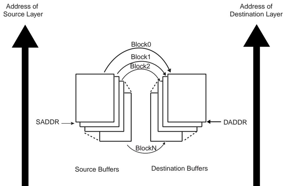
**Figure 40-10. DMAC Transfer Flow for Source and Destination Address Auto-reloaded**
