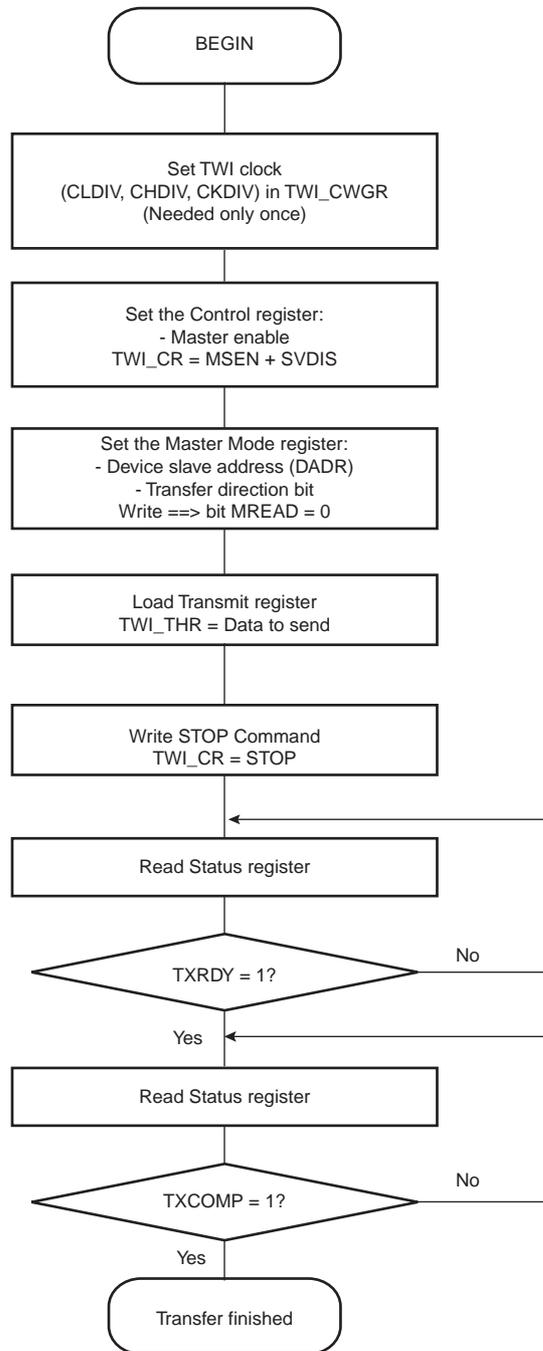
Figure 30-16. TWI Write Operation with Single Data Byte and Internal Address
