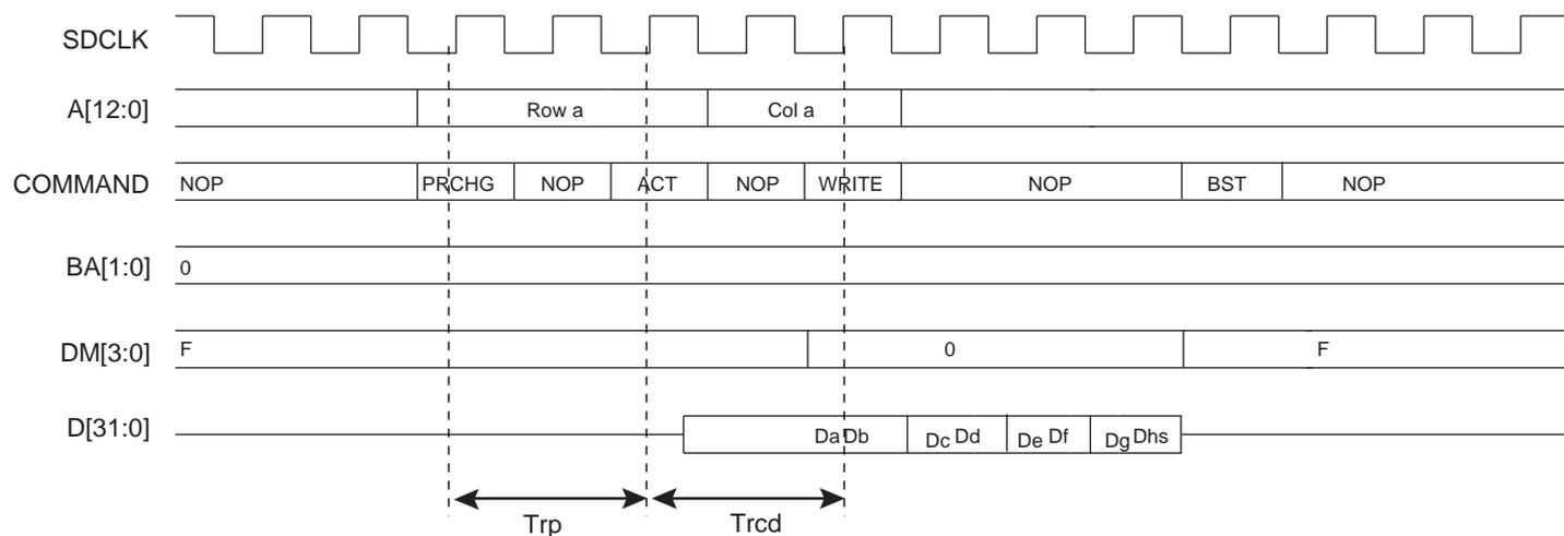
A write command can be followed by a read command. To avoid breaking the current write burst,  $T_{wtr}/T_{wrd} (b/2 + 2 = 6 \text{ cycles})$  should be met. See [Figure 21-8 on page 238](#).
