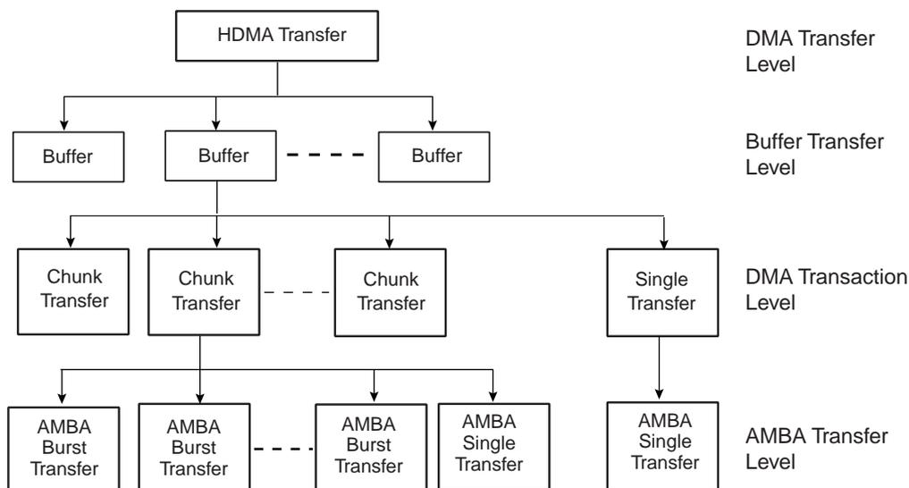
**Figure 40-3. DMAC Transfer Hierarchy for Memory**
