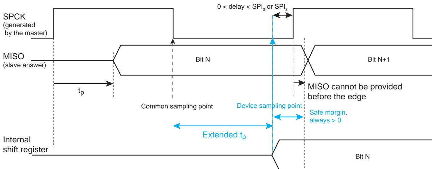
**Figure 48-7. SPI Master Mode 1 and 2**
