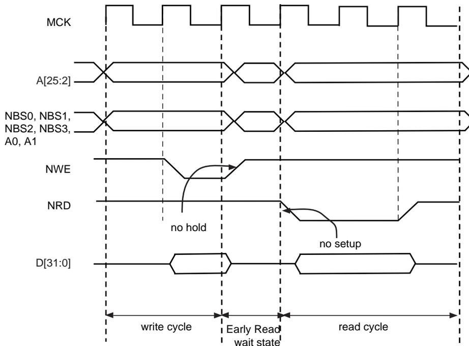
**Figure 20-18. Early Read Wait State: NCS Controlled Write with No Hold Followed by a Read with No NCS Setup**
