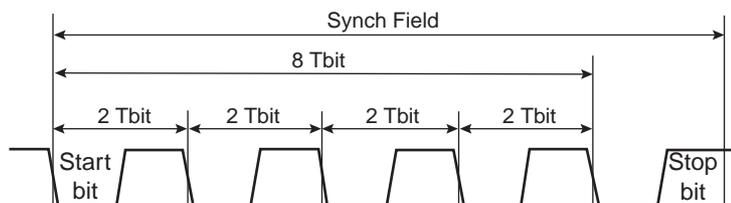
The time measurement is made by a 19-bit counter clocked by the sampling clock (see Section 32.7.1).
