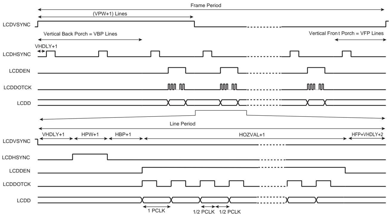
**Figure 47-7. TFT Panel Timing (Line Expanded View), CLKMOD = 1**
