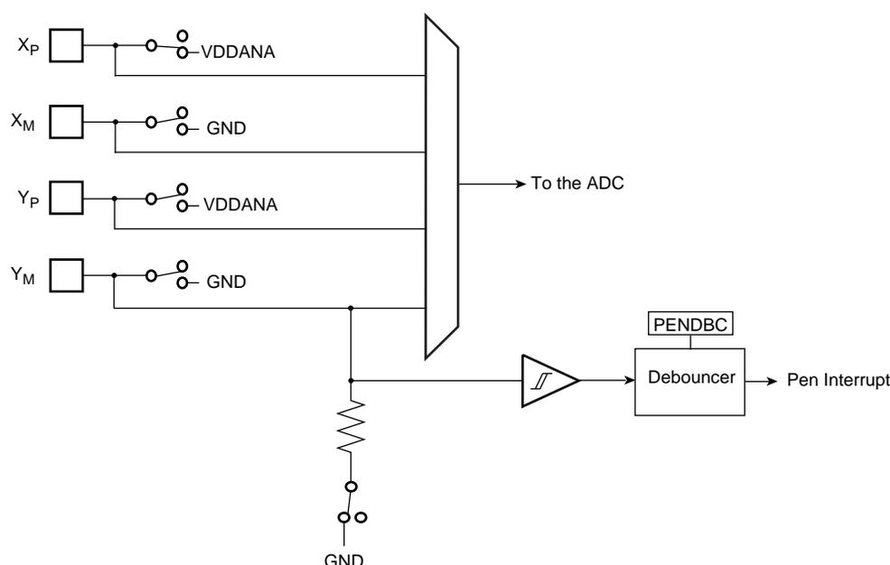
The Touchscreen Pen Detect can be used to generate a TSADCC interrupt to wake up the system or it can be programmed to trig a conversion, so that a position can be measured as soon as a contact is detected if the TSADCC is programmed for an operating mode involving the Touchscreen.
