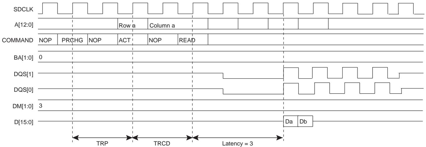
**Figure 21-13. Single Read Access, Row Closed, Latency = 2, SDR-SDRAM Device**
