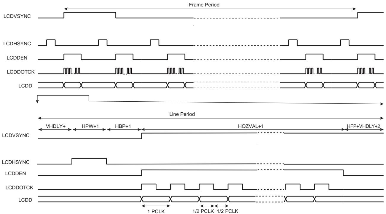
**Figure 47-6. TFT Panel Timing, CLKMOD = 0, VPW = 2, VBP = 2, VFP = 1**
