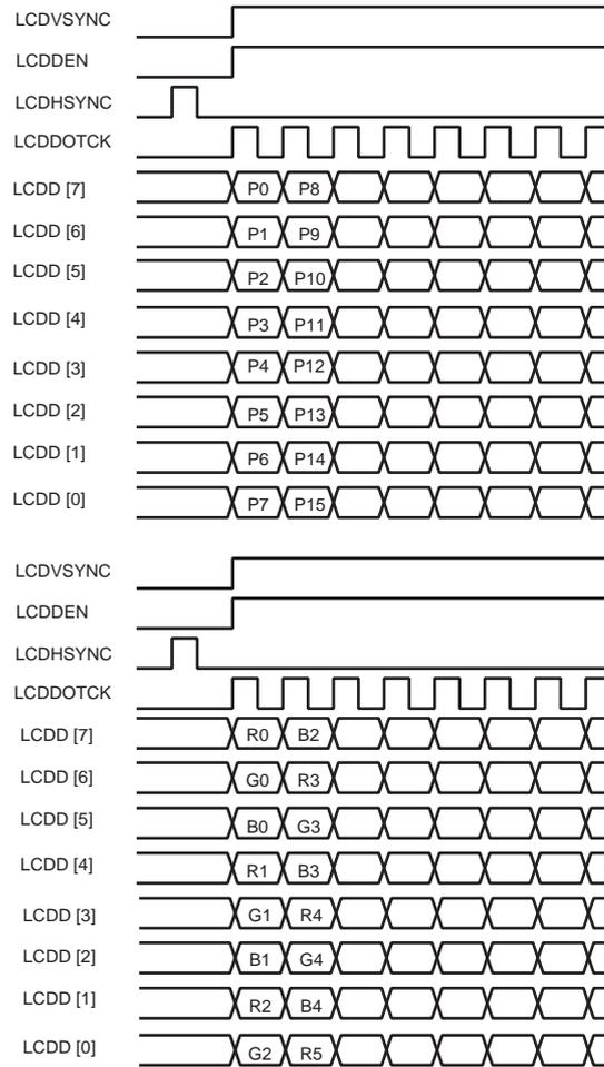
**Figure 47-11. Dual Scan Monochrome and Color 8-bit Panel Timing (First Line Expanded View)**
