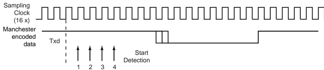
The receiver is activated and starts Preamble and Frame Delimiter detection, sampling the data at one quarter and then three quarters. If a valid preamble pattern or start frame delimiter is detected, the receiver continues decoding with the same synchronization. If the stream does not match a valid pattern or a valid start frame delimiter, the receiver re-synchronizes on the next valid edge. The minimum time threshold to estimate the bit value is three quarters of a bit time.
