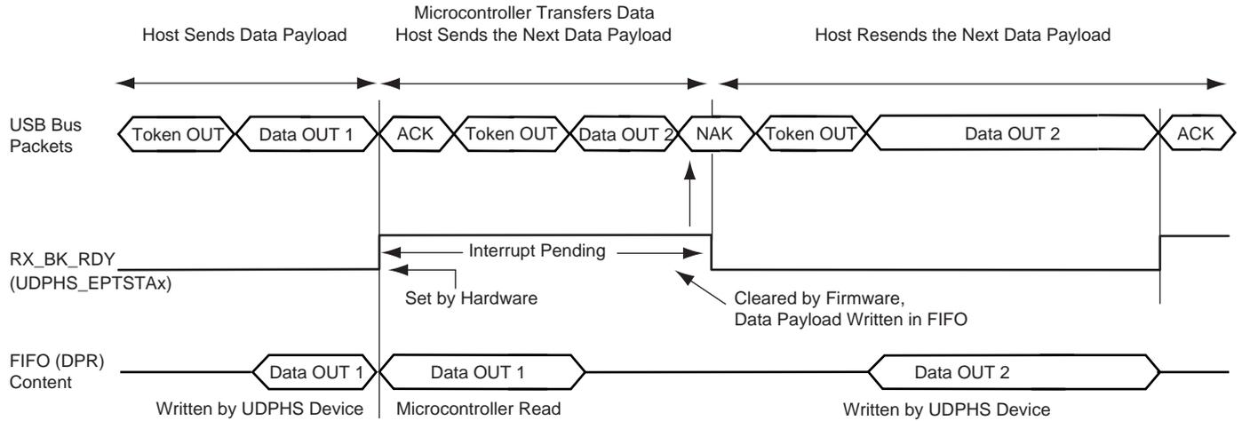
**Figure 37-14. Data OUT Transfer for an Endpoint with Two Banks**
