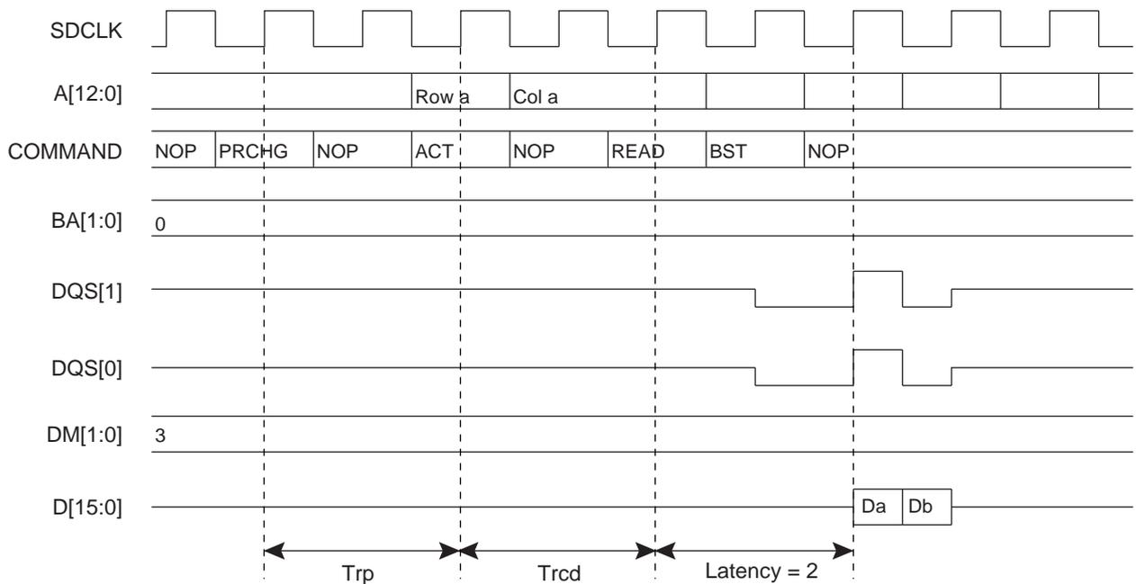
**Figure 21-12. Single Read Access, Row Closed, Latency = 3, DDR2-SDRAM Device**
