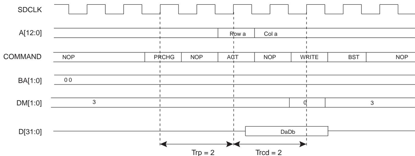
**Figure 21-5. Burst Write Access, Row Closed, Low-power DDR1-SDRAM Device**
