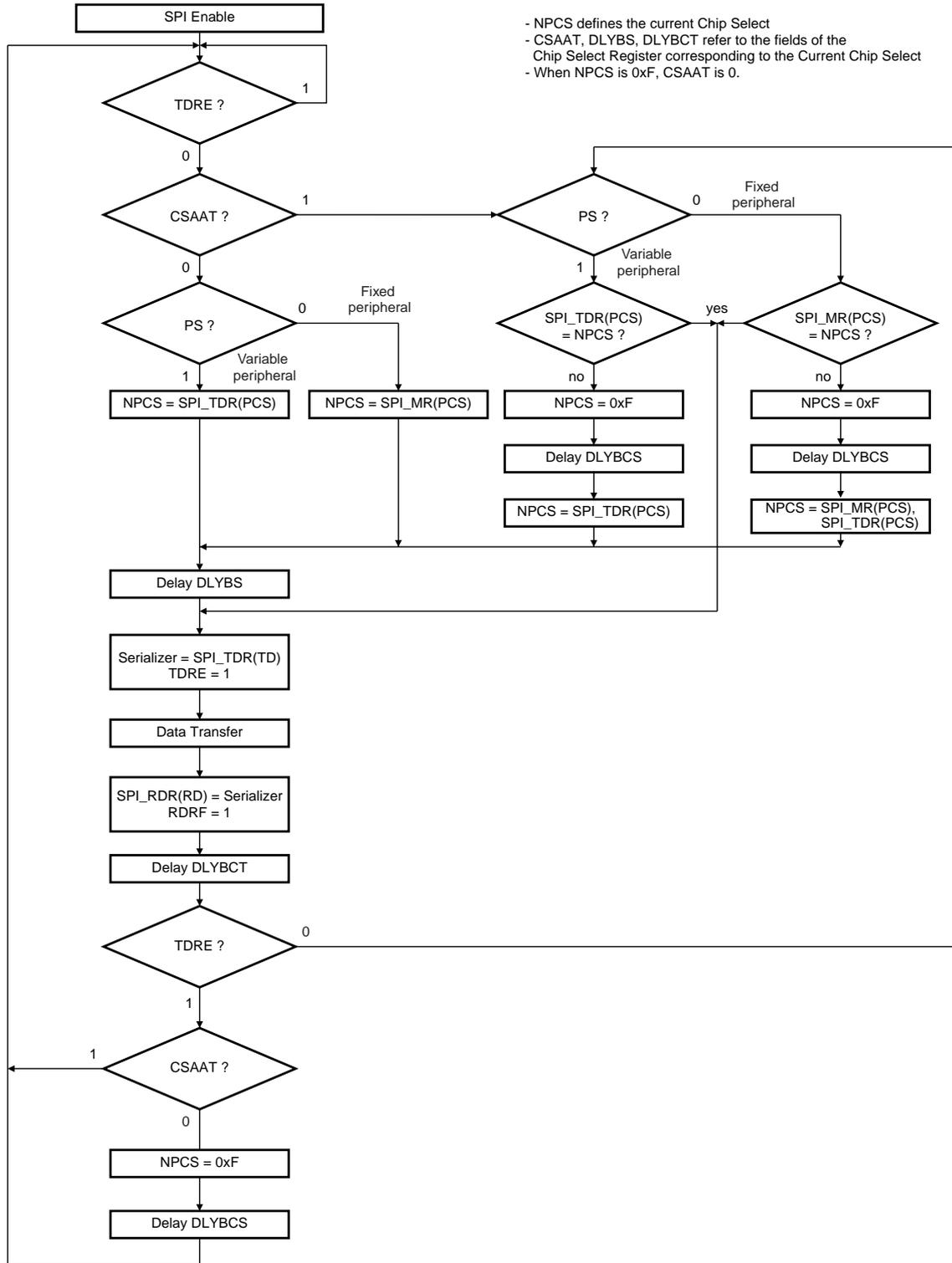
Figure 28-8 shows Transmit Data Register Empty (TDRE), Receive Data Register (RDRF) and Transmission Register Empty (TXEMPTY) status flags behavior within the SPI\_SR (Status Register) during an 8-bit data transfer in fixed mode and no Peripheral Data Controller involved.
