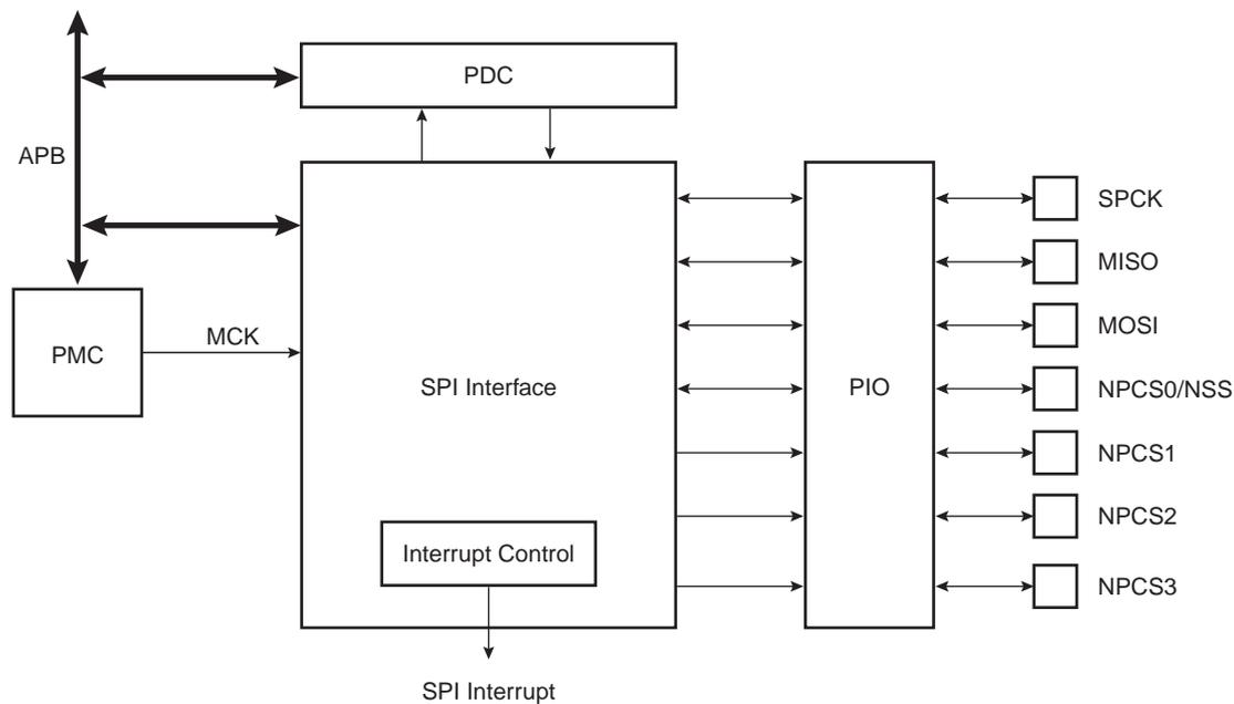
Figure 28-2. Block Diagram
