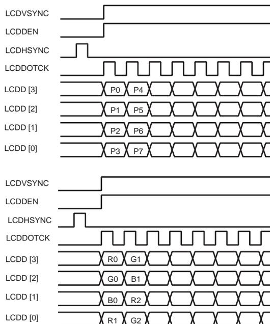
**Figure 47-10. Single Scan Monochrome and Color 8-bit Panel Timing (First Line Expanded View)**
