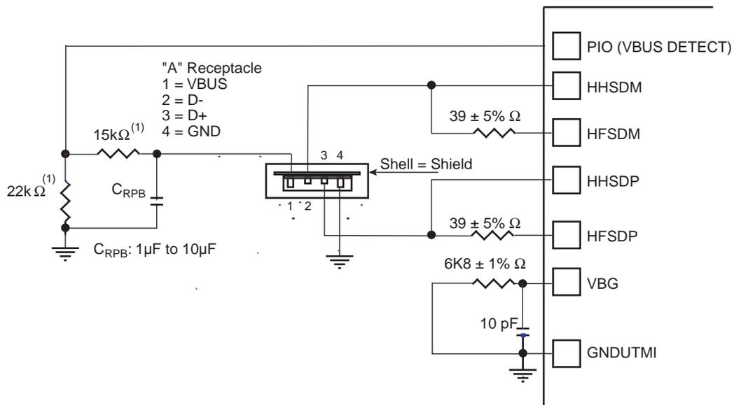
Note: 1. The values shown on the  $22k\Omega$  and  $15k\Omega$  resistors are only valid for 3v3 supplied PIOs.
