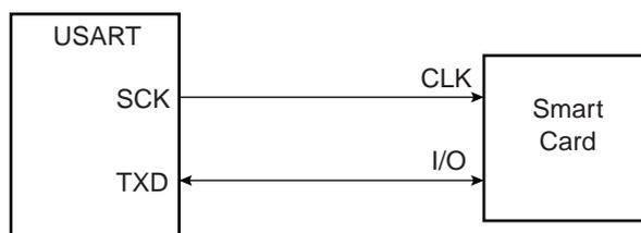
When operating in ISO7816, either in T = 0 or T = 1 modes, the character format is fixed. The configuration is 8 data bits, even parity and 1 or 2 stop bits, regardless of the values programmed in the CHRL, MODE9, PAR and CHMODE fields. MSBF can be used to transmit LSB or MSB first. Parity Bit (PAR) can be used to transmit in normal or inverse mode. Refer to [“USART Mode Register” on page 625](#) and [“PAR: Parity Type” on page 626](#).
