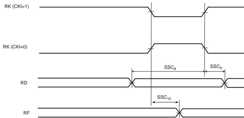
**Figure 48-18. SSC Receiver, RK and RF in Output**
