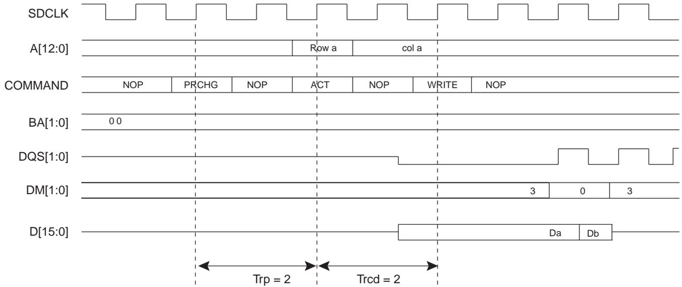
**Figure 21-4. Single Write Access, Row Closed, SDR-SDRAM Device**
