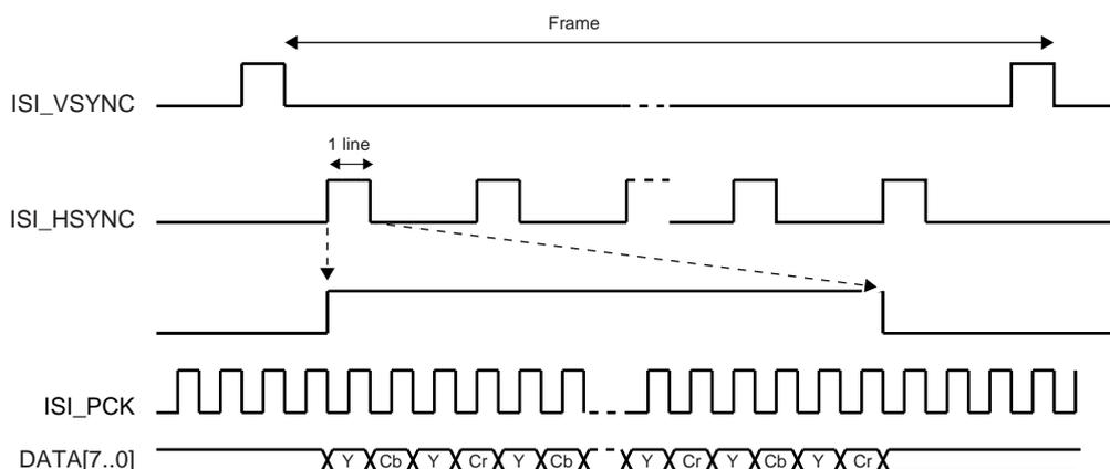
**Figure 38-4. SAV and EAV Sequence Synchronization**
