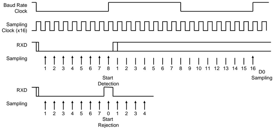
**Figure 32-13. Asynchronous Character Reception**
