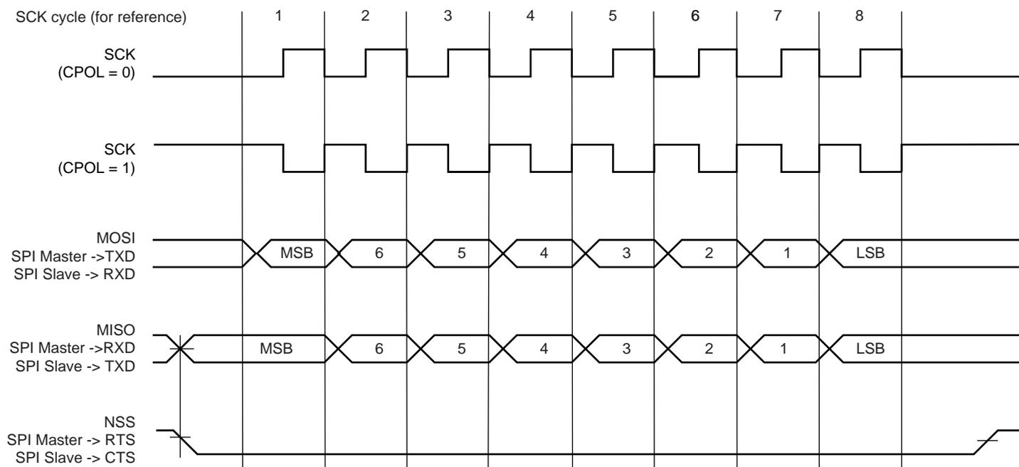
**Figure 32-39. SPI Transfer Format (CPHA = 0, 8 bits per transfer)**
