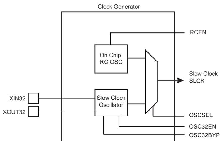
RCEN, OSC32EN, OSCSEL and OSC32BYP bits are located in the Slow Clock Configuration Register (SCKCR) located at address 0xFFFFFD50 in the backed up part of the System Controller and so are preserved while VDDBU is present.
