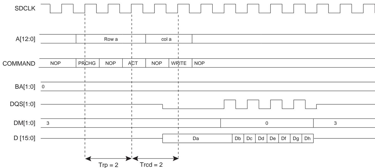
**Figure 21-7. Burst Write Access, Row Closed, SDR-SDRAM Device**
