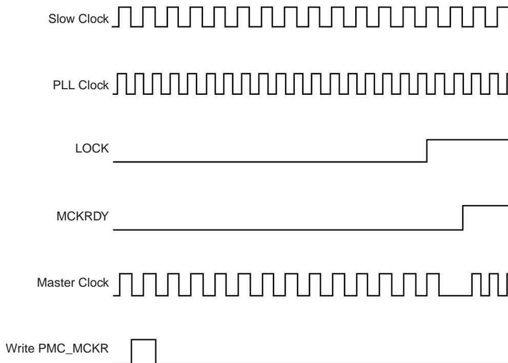
**Figure 25-4. Switch Master Clock from Main Clock to Slow Clock**
