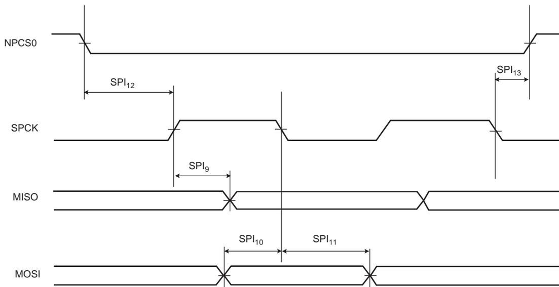
**Figure 48-11. SPI Slave Mode - NPCS Timings**
