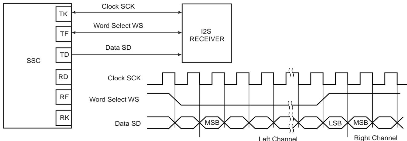
**Figure 33-20. Codec Application Block Diagram**
