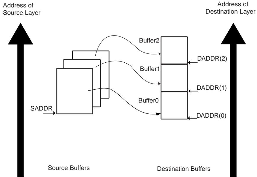
**Figure 40-14. DMAC Transfer Replay Mode is Enabled for the Source and Contiguous Destination Address**
