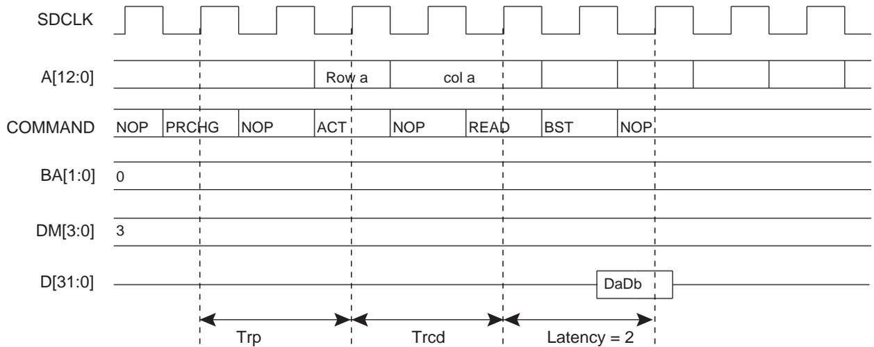
**Figure 21-14. Burst Read Access, Latency = 2, Low-power DDR1-SDRAM Devices**
