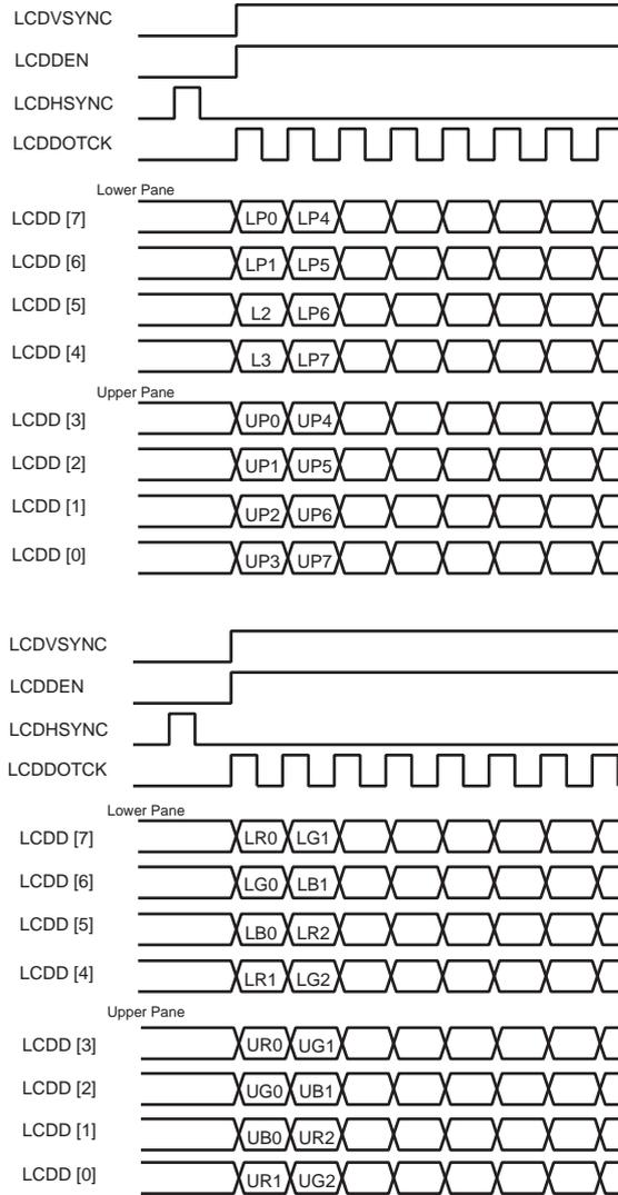
**Figure 47-12. Dual Scan Monochrome and Color 16-bit Panel Timing (First Line Expanded View)**
