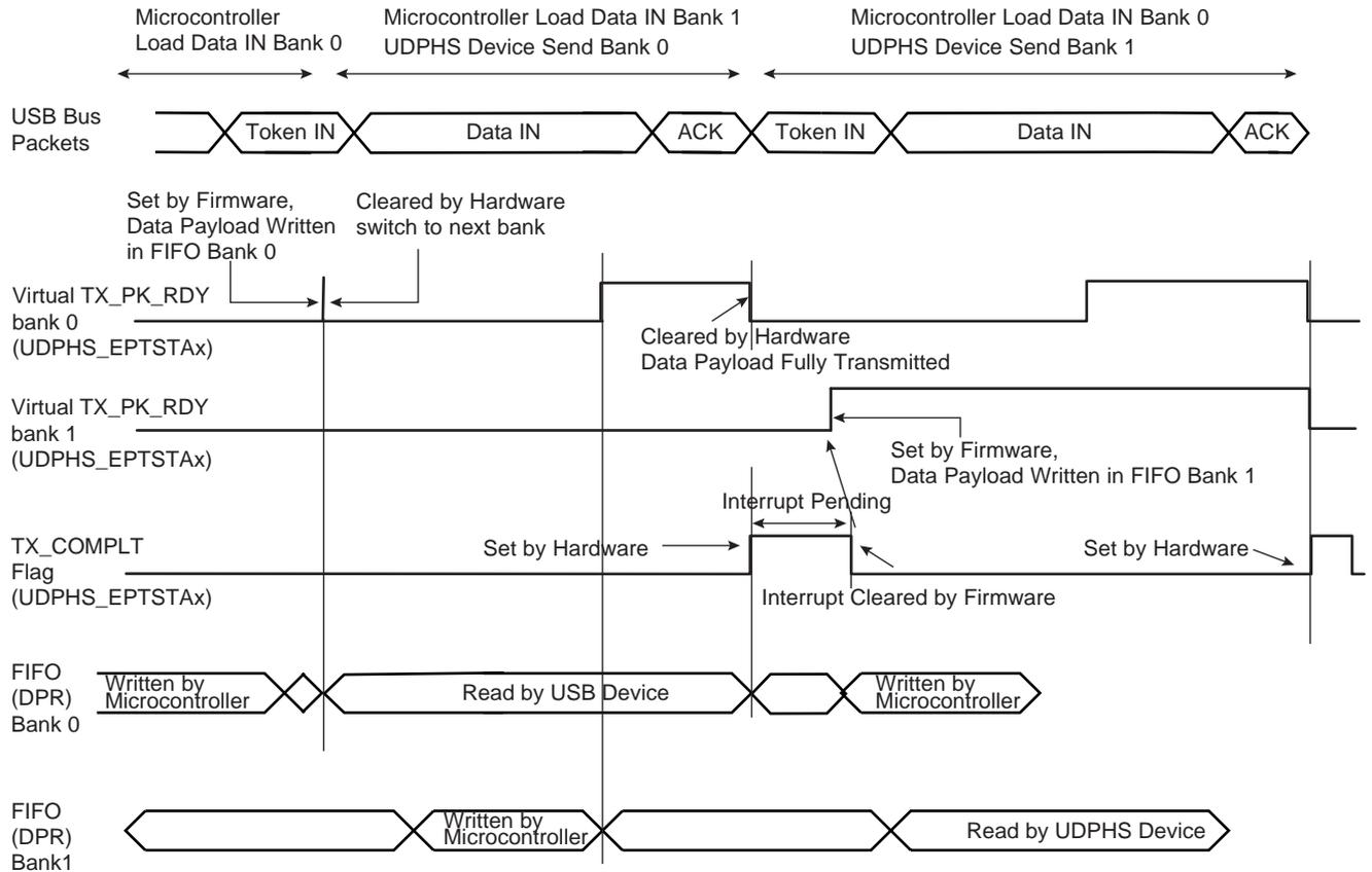
**Figure 37-10. Data IN Followed By Status OUT Transfer at the End of a Control Transfer**
