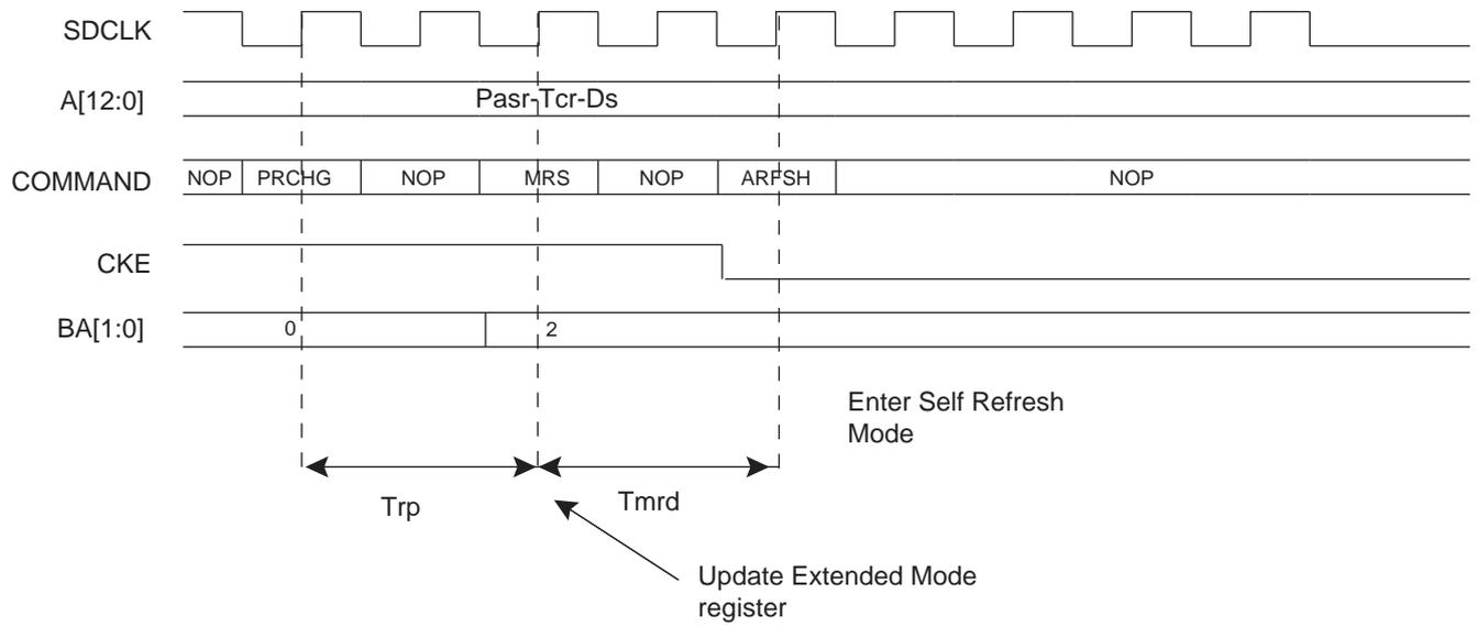
**Figure 21-21. Automatic Update During AUTO-REFRESH Command and SDRAM Access**
