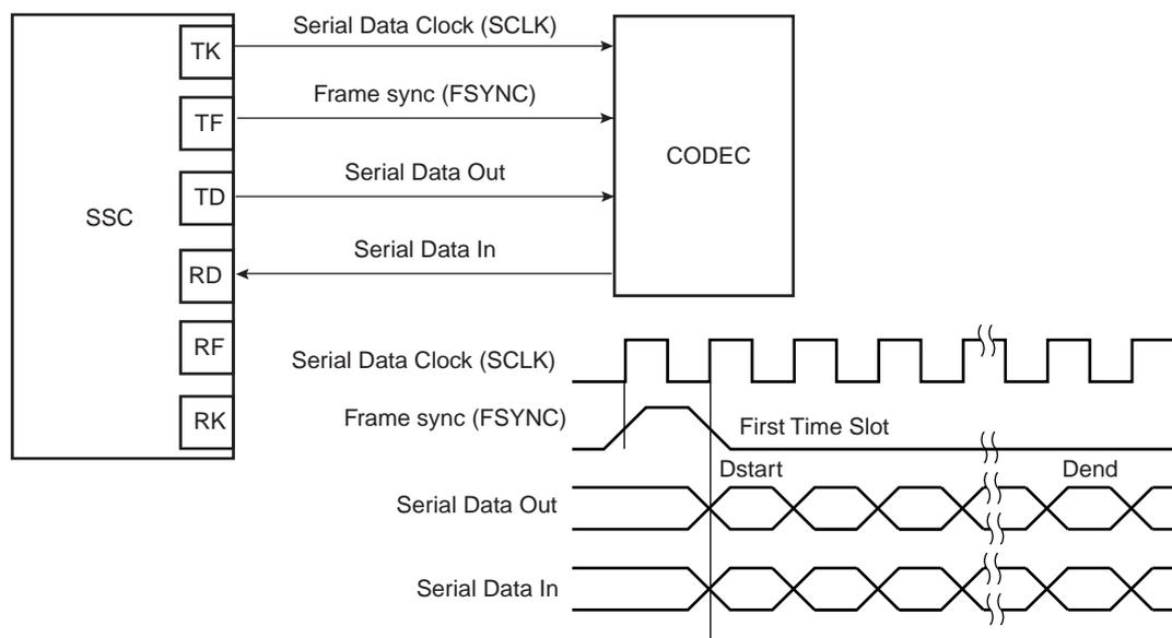
**Figure 33-21. Time Slot Application Block Diagram**
