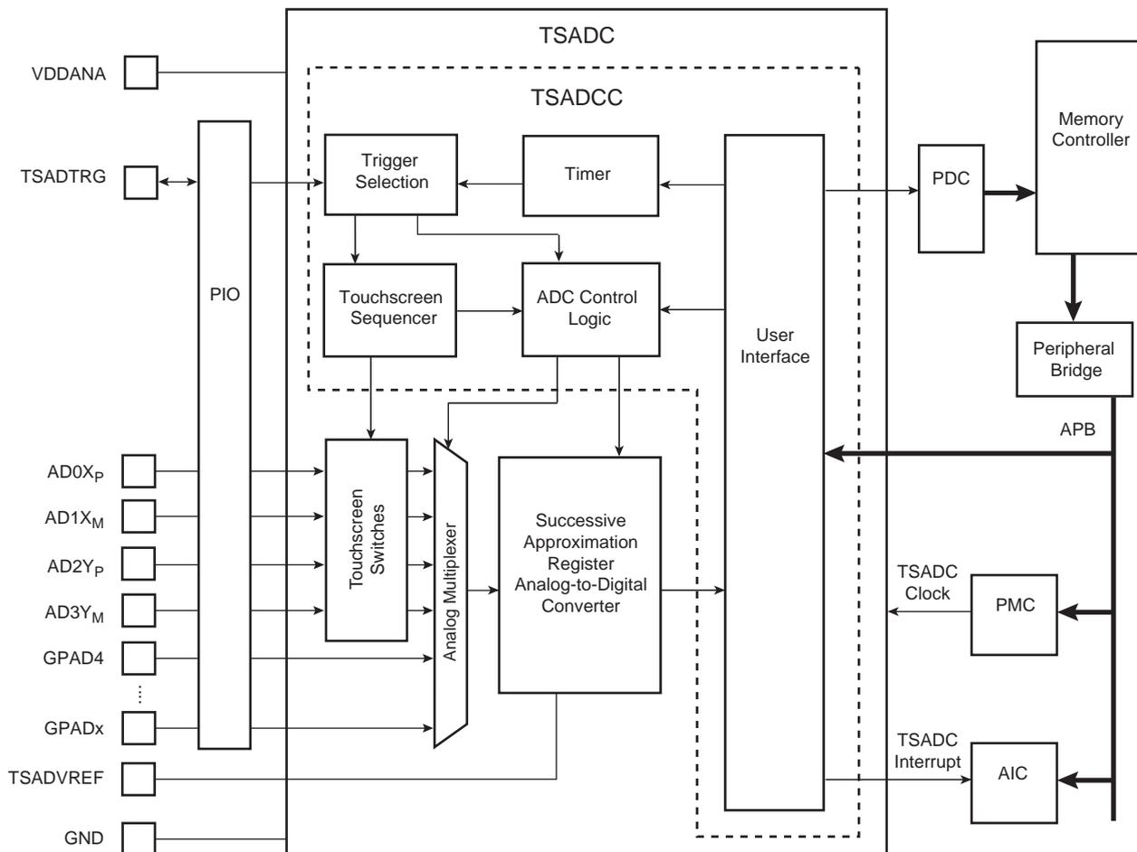
GPADx: last general-purpose ADC channel defined by the number of channels
