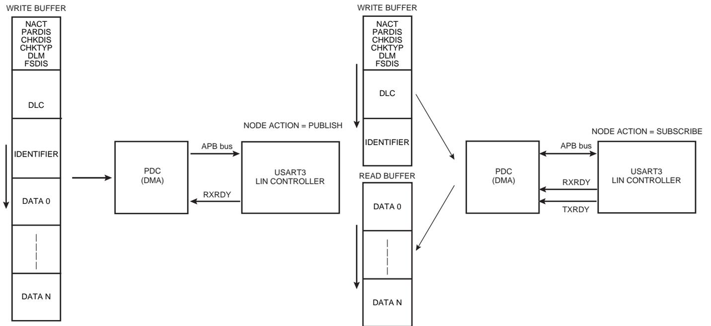
**Figure 32-53. Master Node with PDC (PDCM = 0)**
