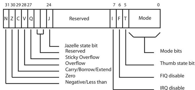
Figure 8-2 shows the status register format, where:
