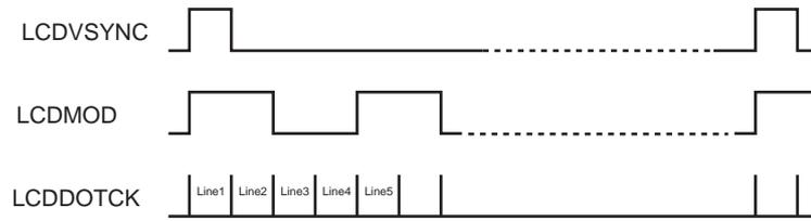
**Figure 47-4. Full Frame Timing, MMODE = 0**
