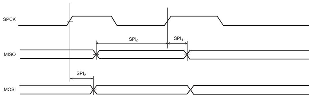
**Figure 48-8. SPI Master Mode 0 and 3**
