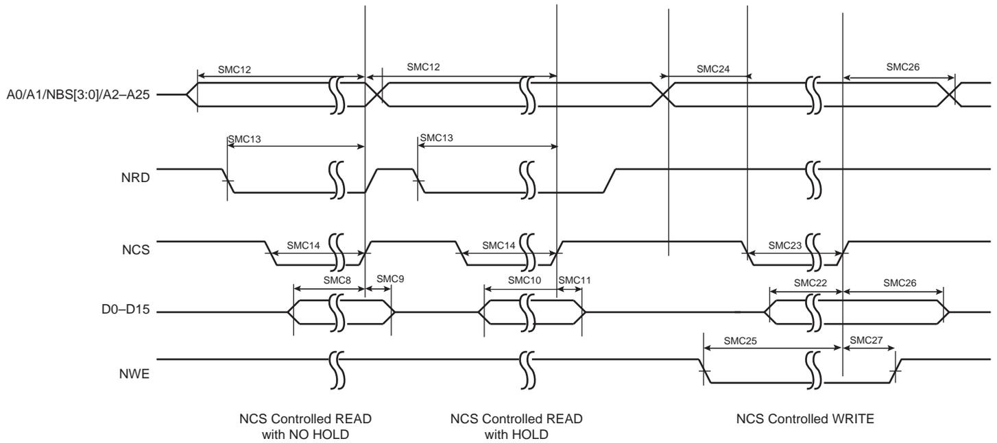
**Figure 48-5. SMC Timings - NRD Controlled Read and NWE Controlled Write**
