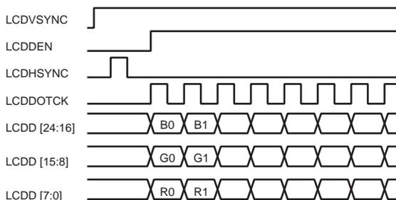
**Figure 47-9. Single Scan Monochrome and Color 4-bit Panel Timing (First Line Expanded View)**
