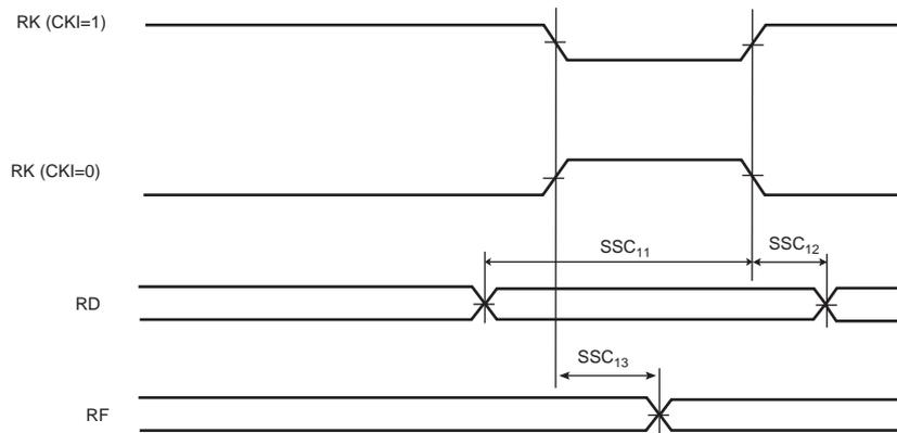
**Figure 48-19. SSC Receiver, RK in Output and RF in Input**
