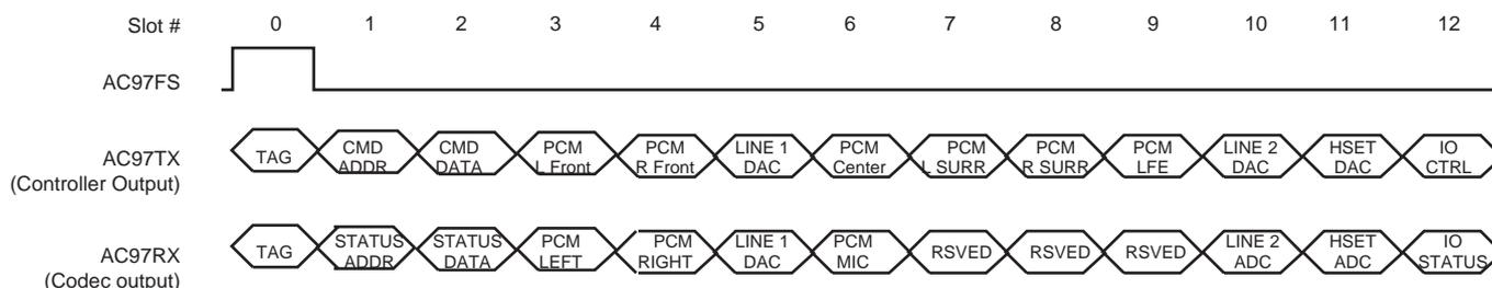
**Table 42-4. AC-link Output Slots Transmitted from the AC97C Controller**
