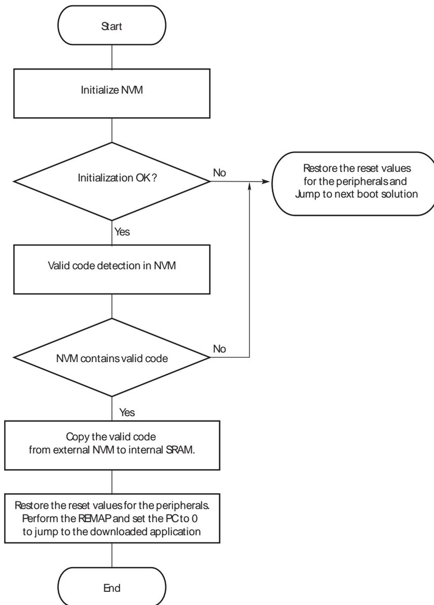
**Figure 10-3. Remap Action after Download Completion**
