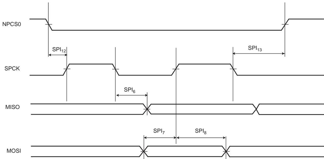
**Figure 48-10. SPI Slave Mode 1 and 2**
