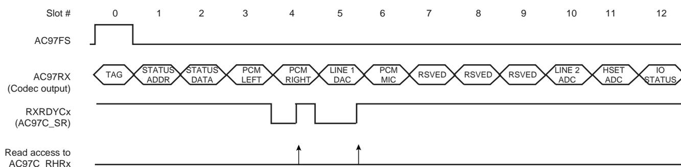
If the previously received data has not been read by the application, the new data overwrites the data already waiting in AC97C\_CxRHR, therefore the OVRUN flag in AC97C\_CxSR is raised. The application can either poll the OVRUN flag in AC97C\_CxSR or wait for an interrupt notice. The interrupt remains active until the OVRUN flag in AC97C\_CxSR is set.
