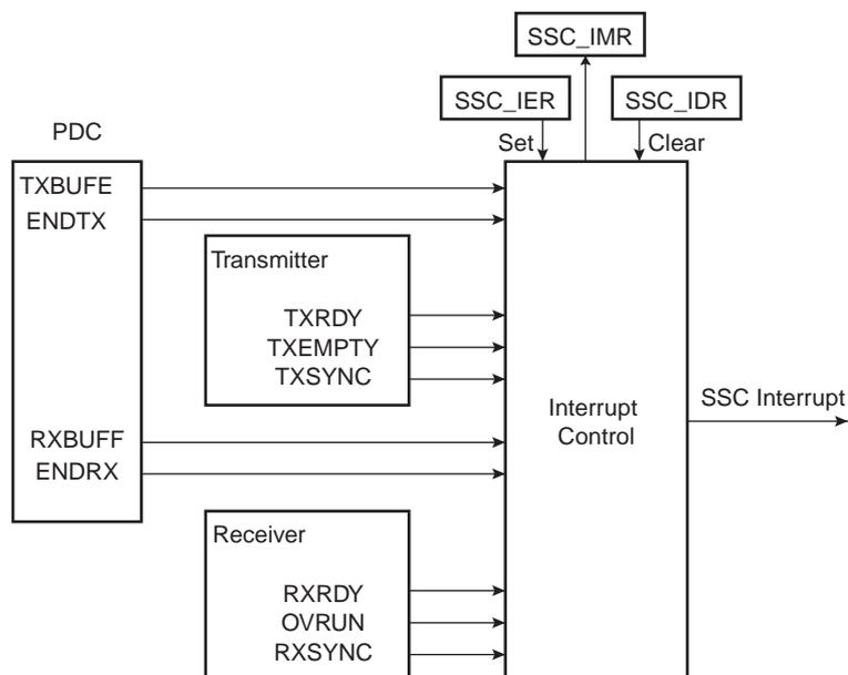
Figure 33-18. Interrupt Block Diagram (with DMA)
