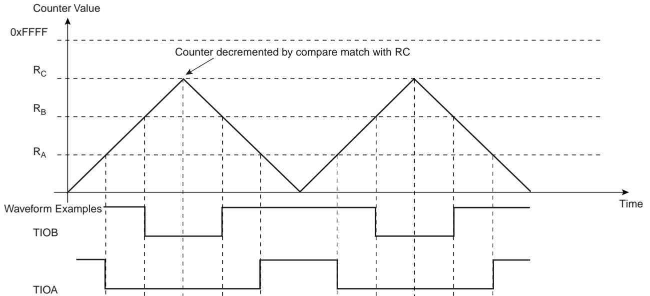
**Figure 31-14. WAVSEL = 11 With Trigger**
