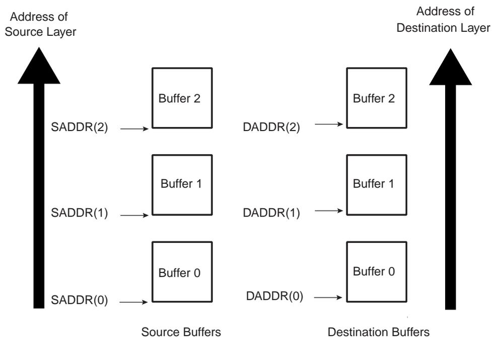
If the user needs to execute a DMAC transfer where the source and destination address are contiguous but the amount of data to be transferred is greater than the maximum buffer size DMAC\_CTRLAx.BTSIZE, then this can be achieved using the type of multi-buffer transfer as shown in [Figure 40-7](#).
