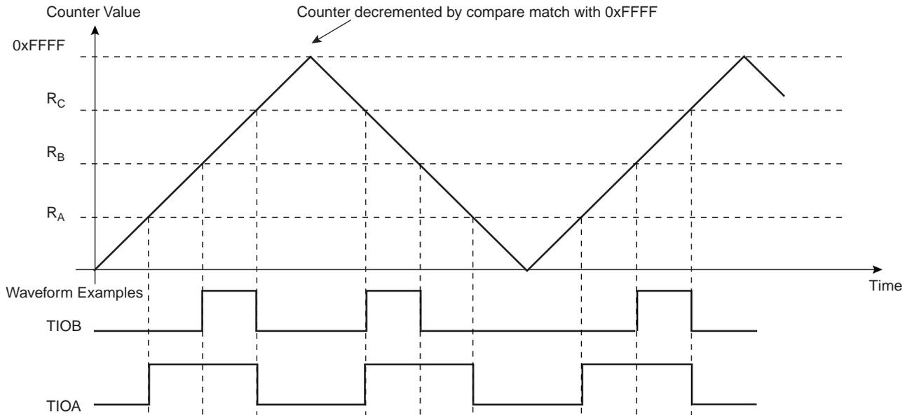
**Figure 31-12. WAVSEL = 01 With Trigger**
