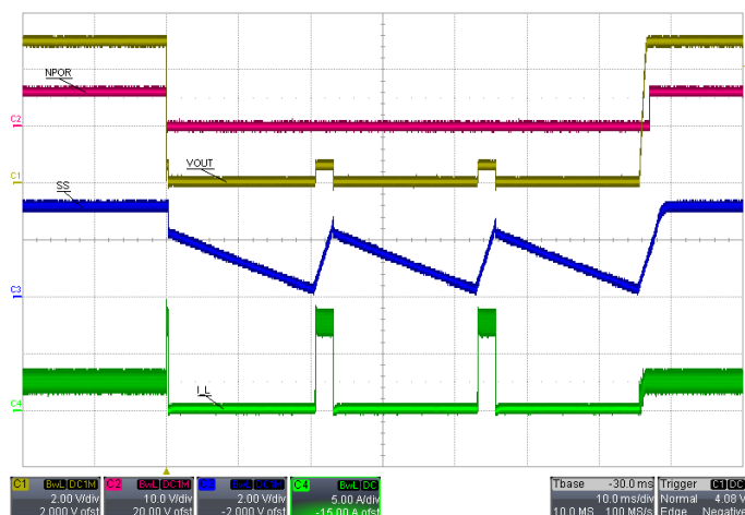
Figure 12: Hiccup Mode Protection and Recovery
