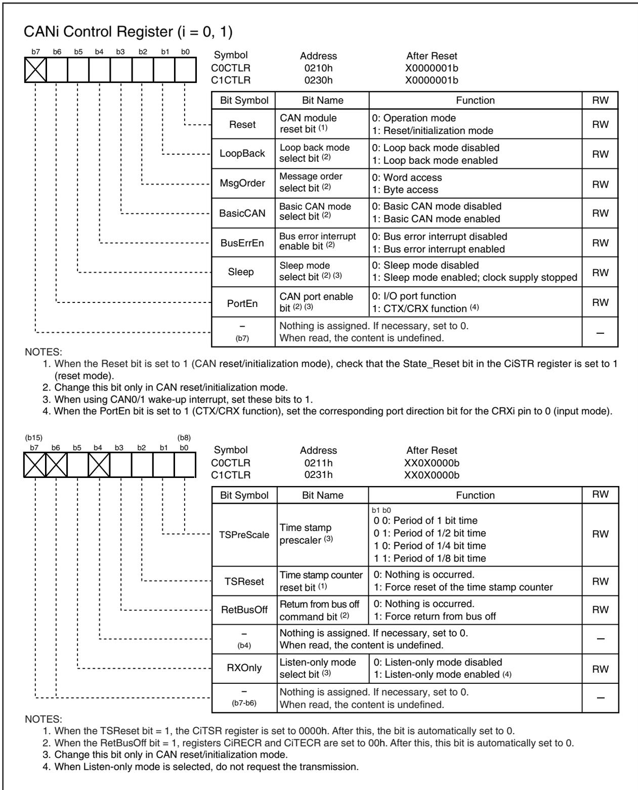
**Figure 19.7 Registers C0CTLR and C1CTLR**
