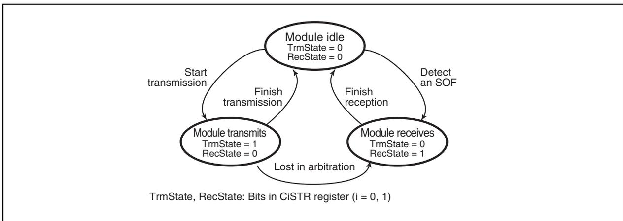
Figure 19.13 Sub Modes of CAN Operation Mode
