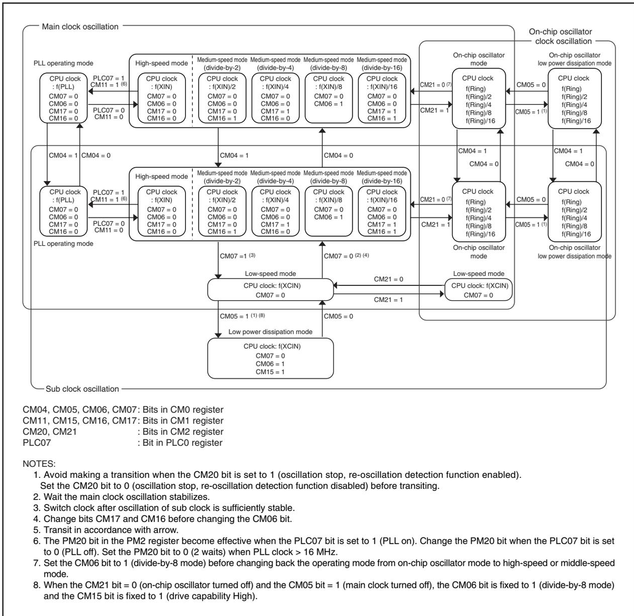
Figure 8.13 State Transition in Normal Operating Mode
