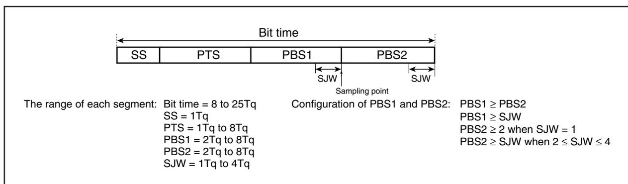
**Figure 19.15 Bit Timing**
