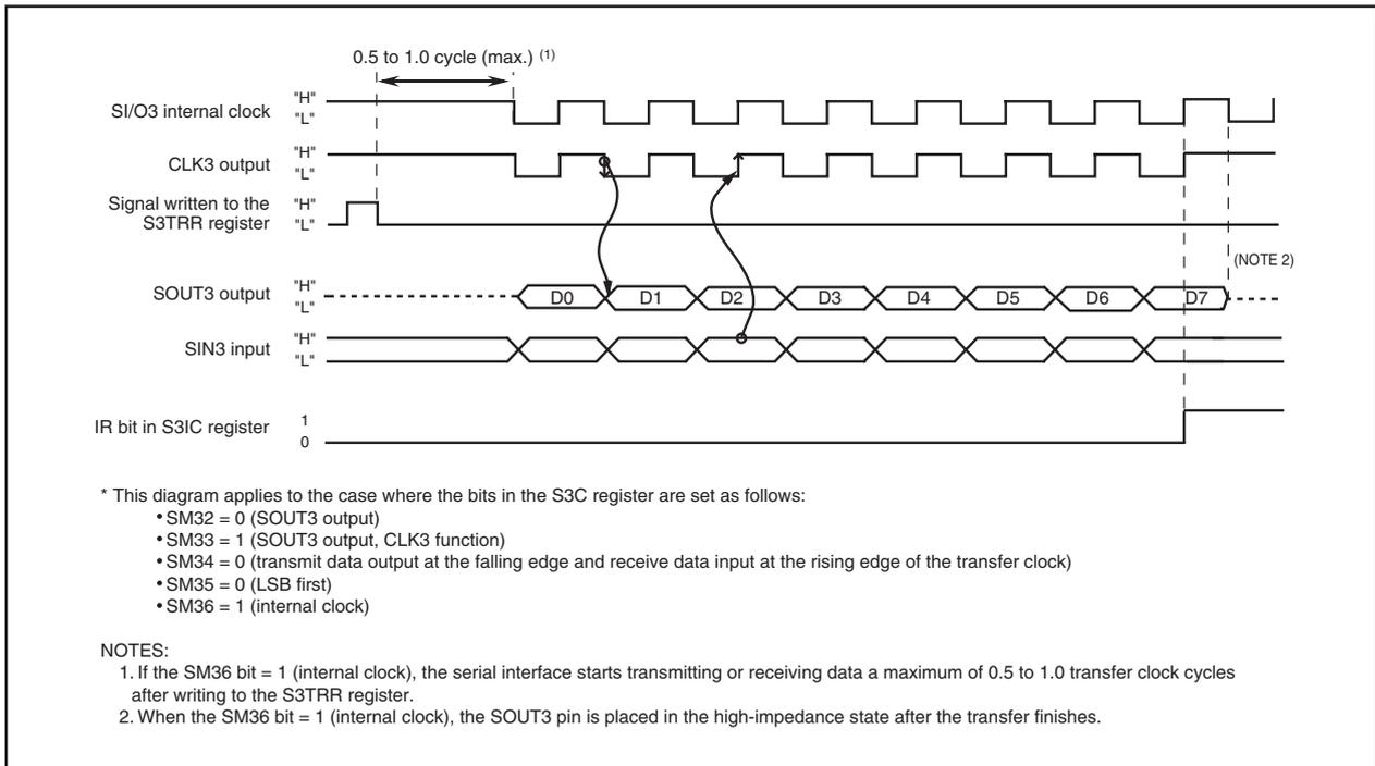
Figure 15.38 SI/O3 Operation Timing
