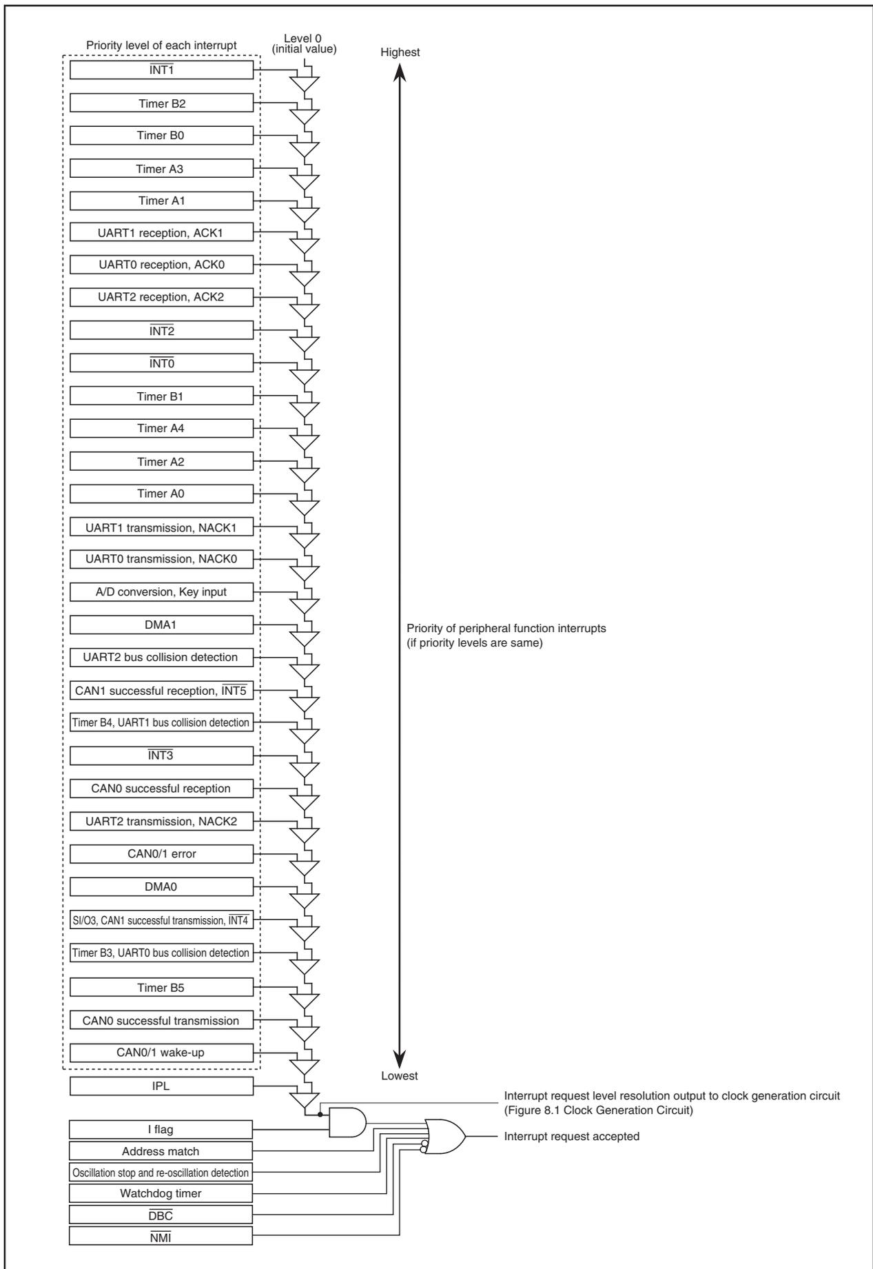
Figure 10.10 Interrupts Priority Select Circuit
