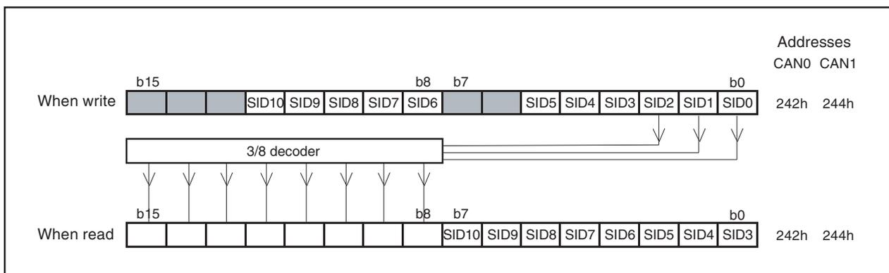
**Figure 19.18 Write/read of CiAFS Register in Word Access**
