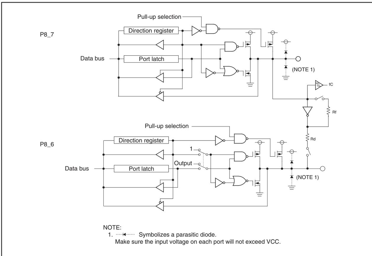
Figure 20.5 I/O Ports (5)
