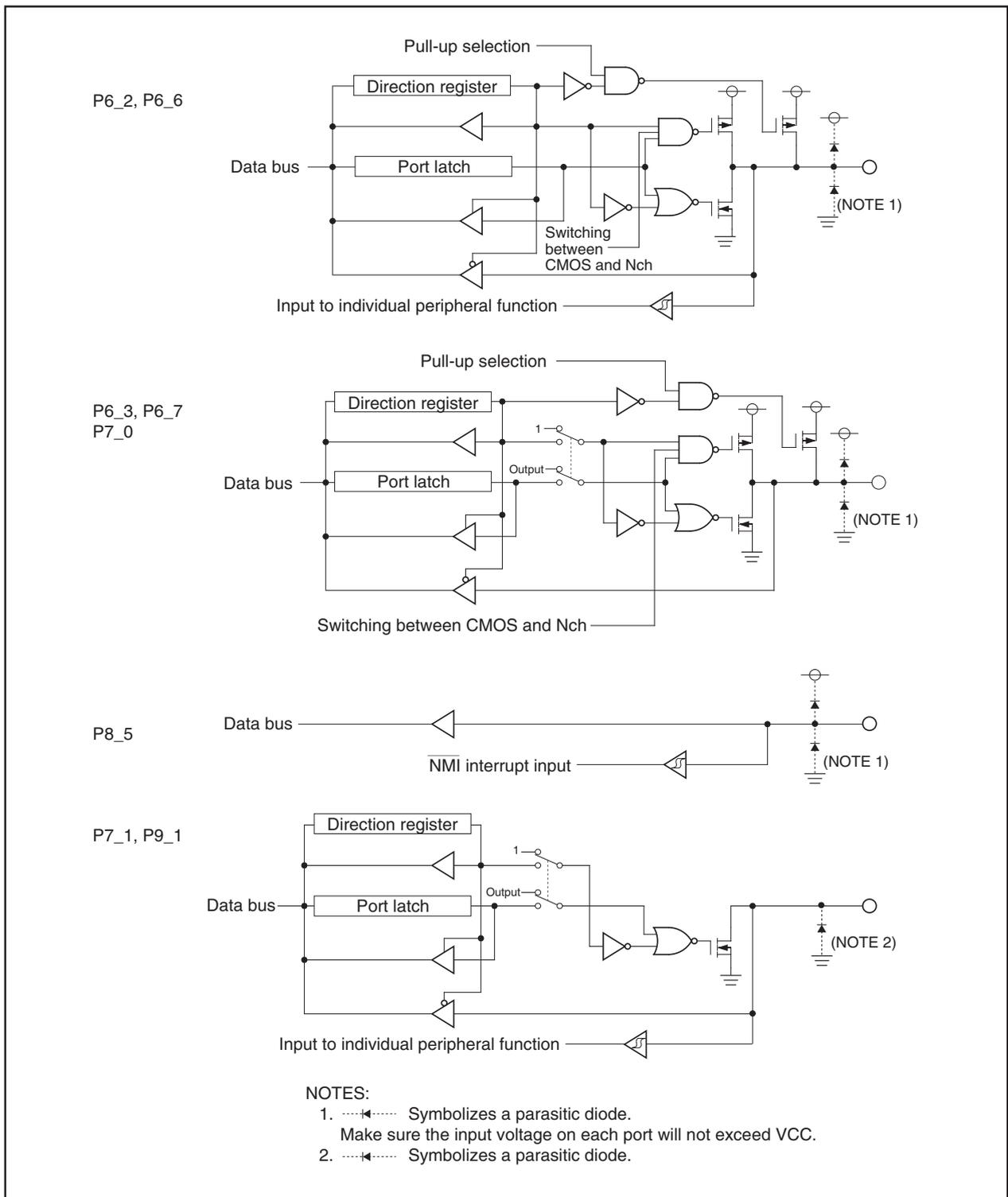
Figure 20.3 I/O Ports (3)
