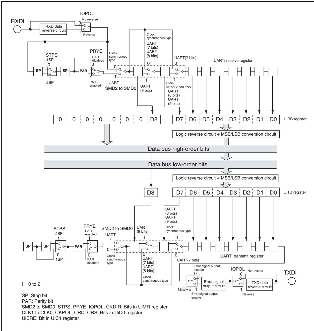
Figure 15.4 UARTi Transmit/Receive Unit
