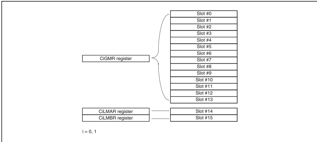
**Figure 19.16** Correspondence of Mask Registers to Slots
