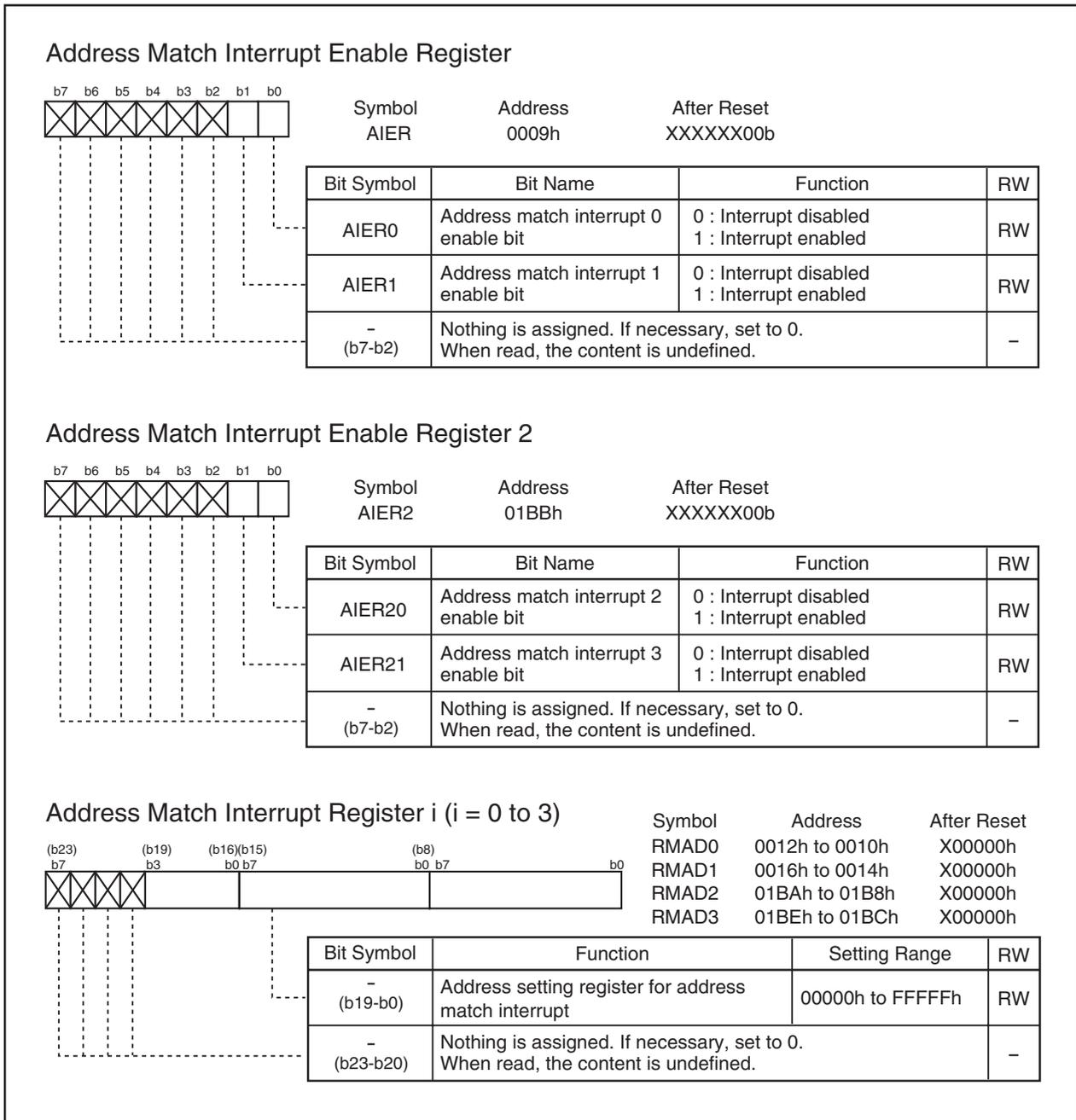
Figure 10.14 Registers AIER, AIER2, and RMAD0 to RMAD3
