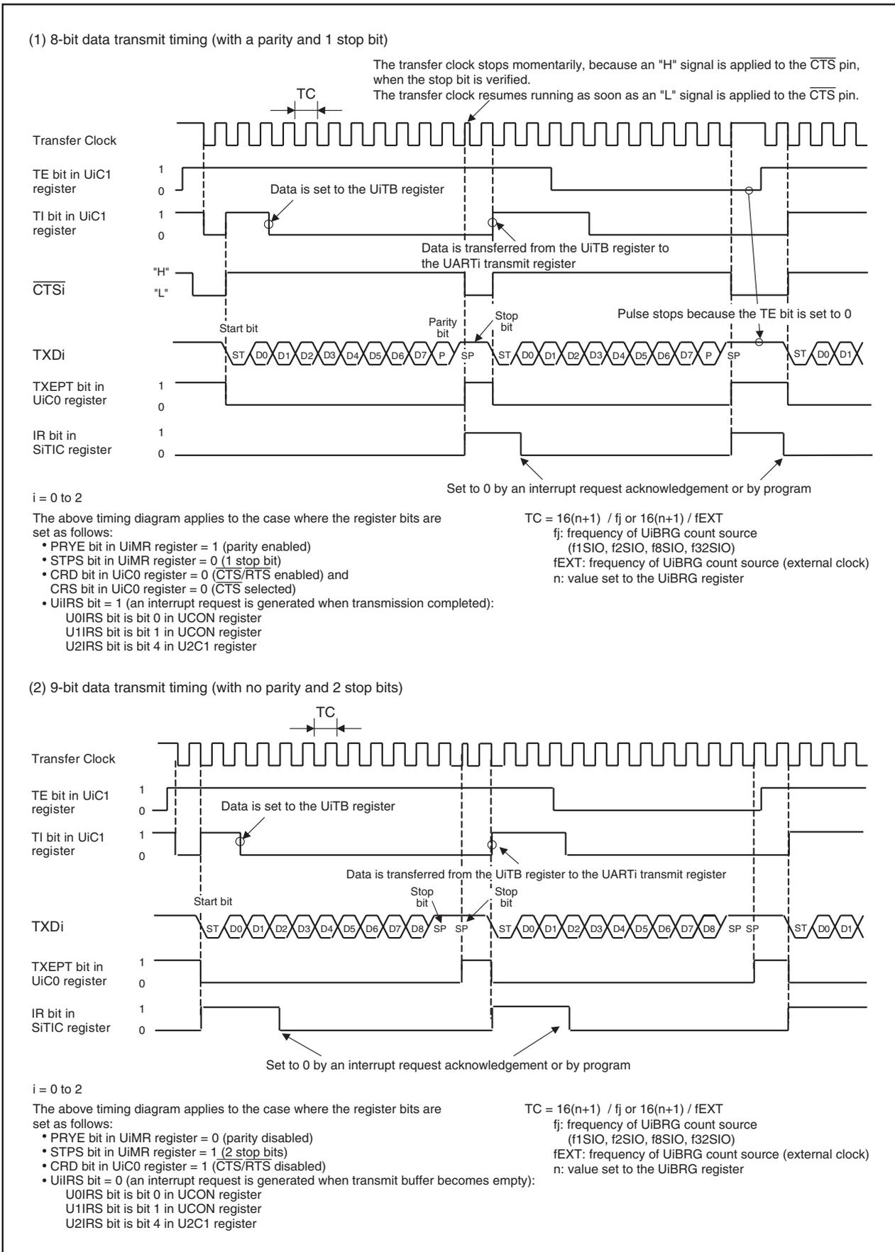
Figure 15.17 Transmit Operation
