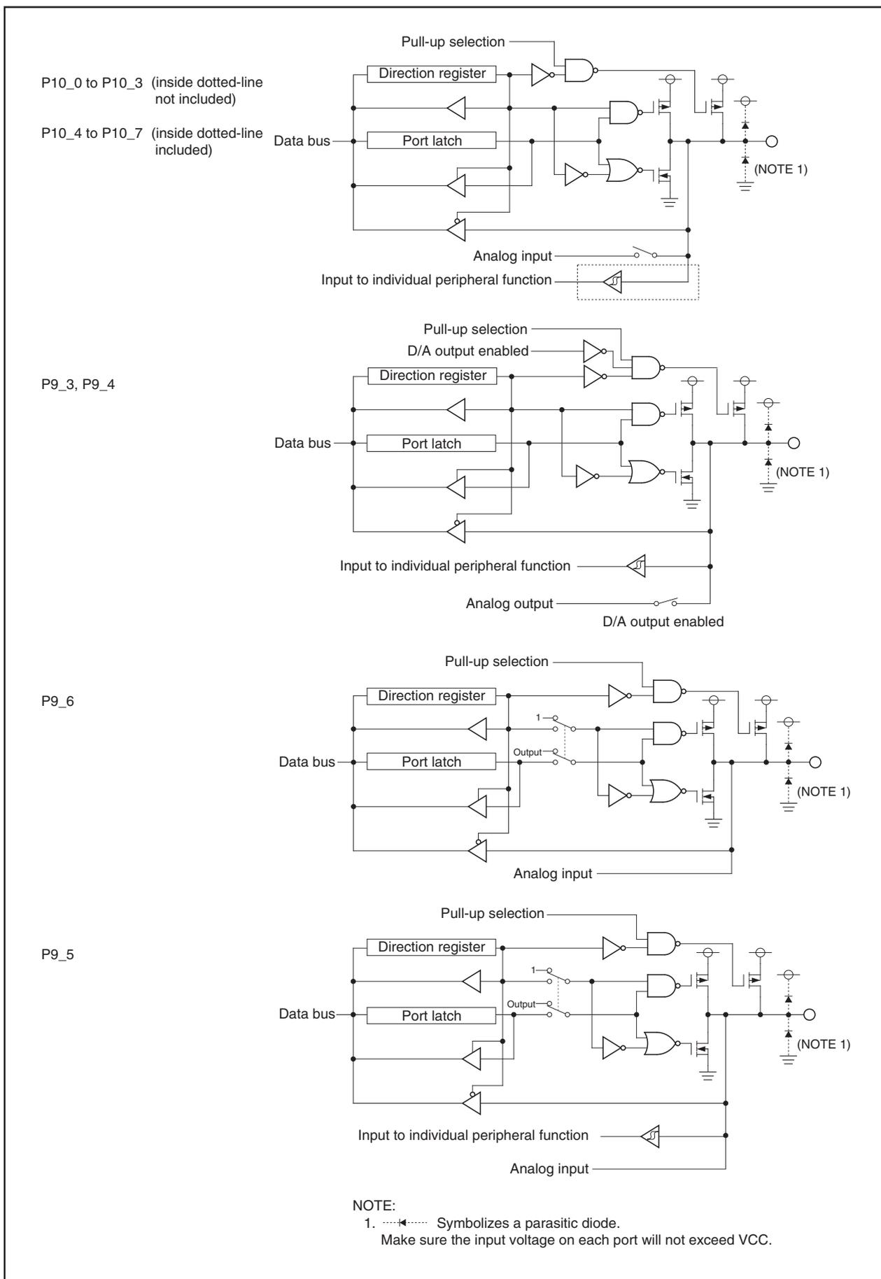
Figure 20.4 I/O Ports (4)
