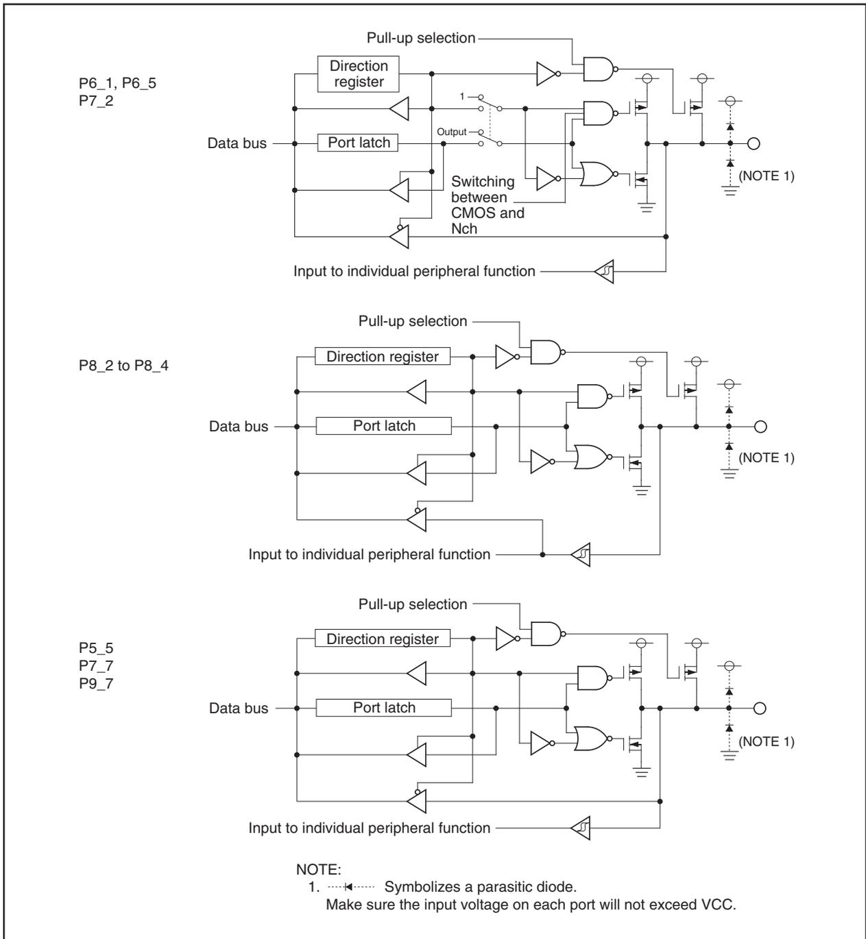
Figure 20.2 I/O Ports (2)
