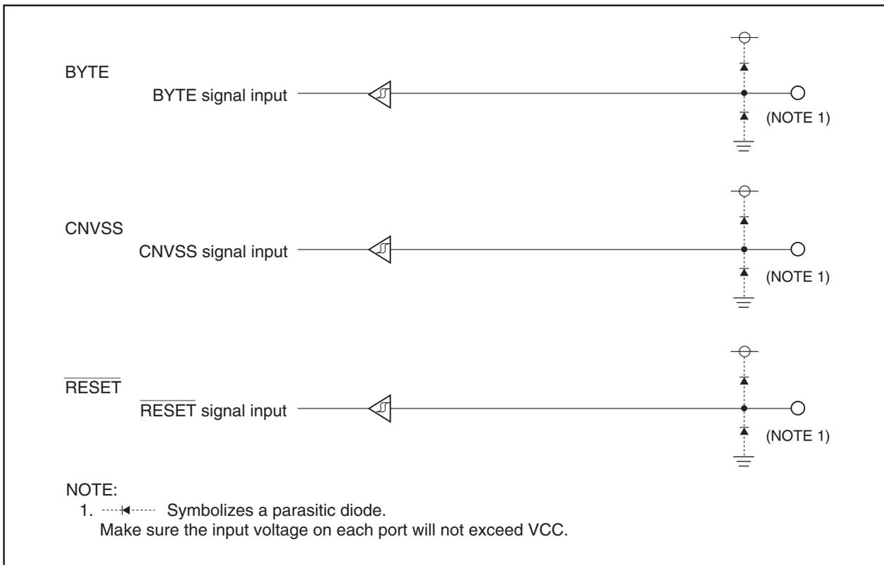
Figure 20.6 I/O Pins
