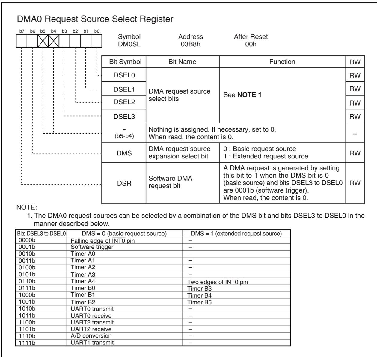
**Figure 12.2 DM0SL Register**
