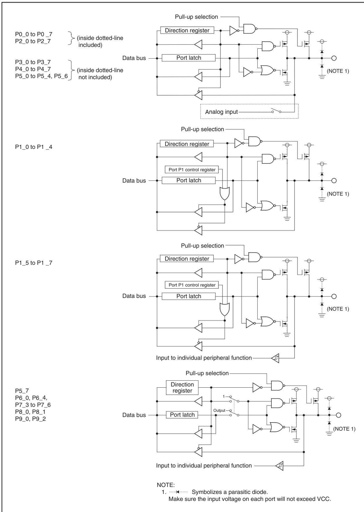
Figure 20.1 I/O Ports (1)
