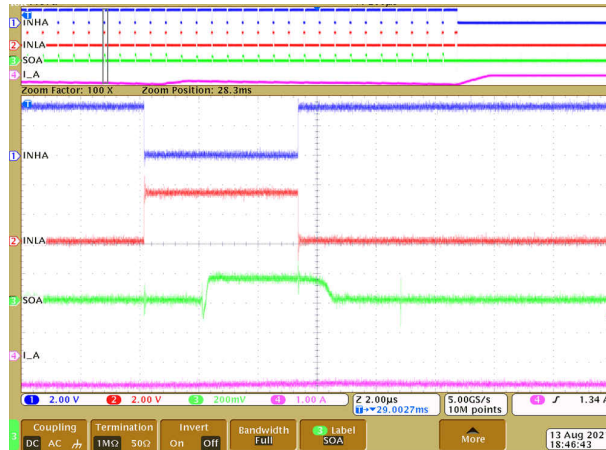
Figure 9-6. Driver PWM operation with feedback
