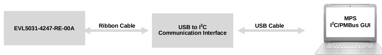
Figure 1: EVKT-MP5031 Evaluation Kit Set-Up
