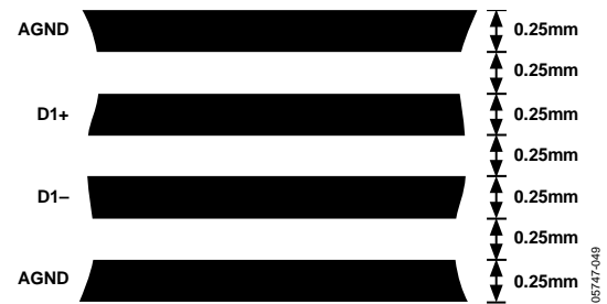
Figure 61. Arrangement of Signal Tracks
