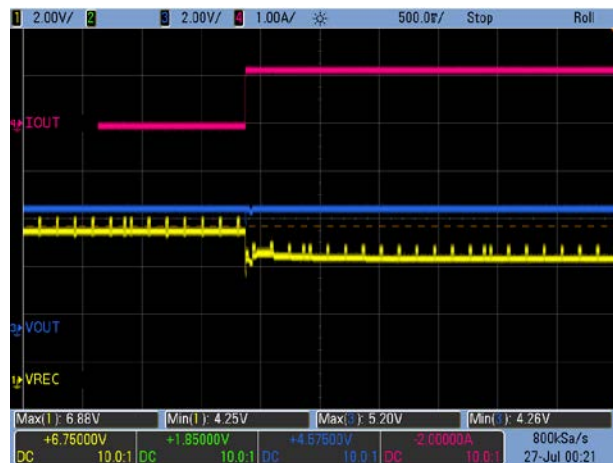
Figure 11. Load Transient: V_{OUT} = 5V , 0A \rightarrow 1.2A
